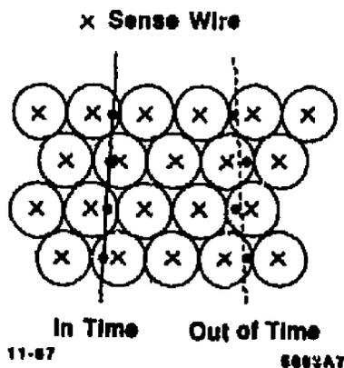
Fig. 1. Layers of straw tubes in a superlayer with every other layer staggered by the straw tube radius. A single in-time track will appear as a series of hits on the wires on alternate sides of the track. The left-right ambiguity is easily resolved locally. A track from an out-of-time bunch crossing will produce hits which are displaced from possible tracks by at least 16 ns in drift time.
