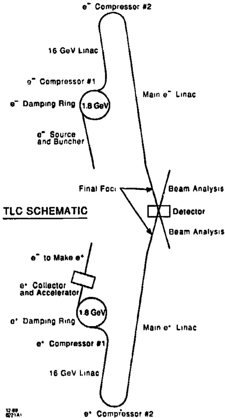
Fig. 1. Schematic layout of an ILC or TLC. The angles shown are exaggerated.
