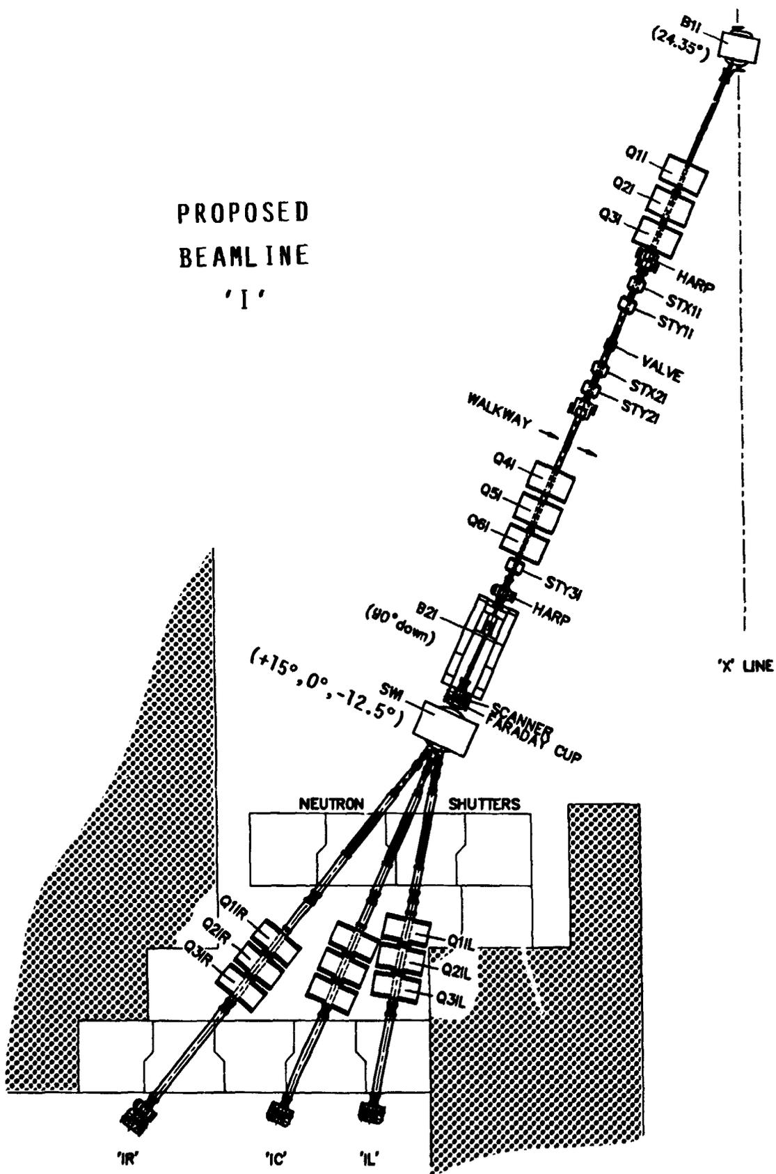
Fig. 5 Diagram of the revised isotope production beamlines, incorporating quadrupole triplets on each line after the switching magnet.
