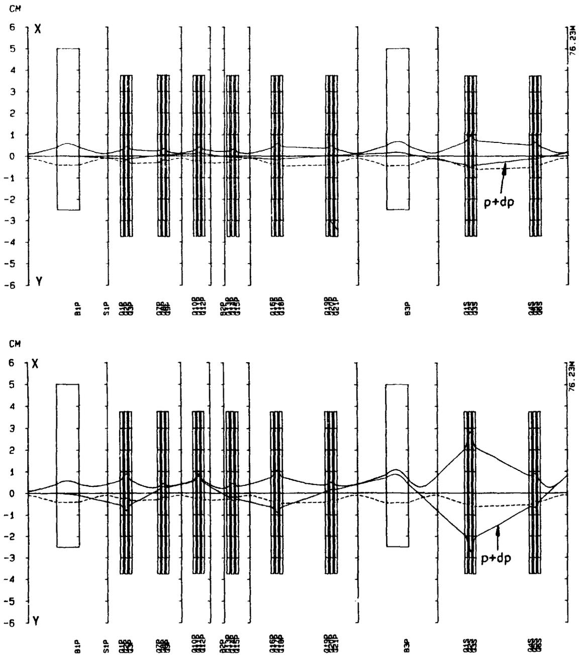
Fig. 6 Beam envelope plots for the double-monochromator and 2-triplet quadrupole matching system leading to the spectrometer target, for 0.1% (top) and 0.5% momentum spread (below).
