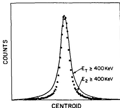
Fig. 3. Typical centroid spectrum without suppression of events from Compton scattering (solid curve) and with such suppression (points)
