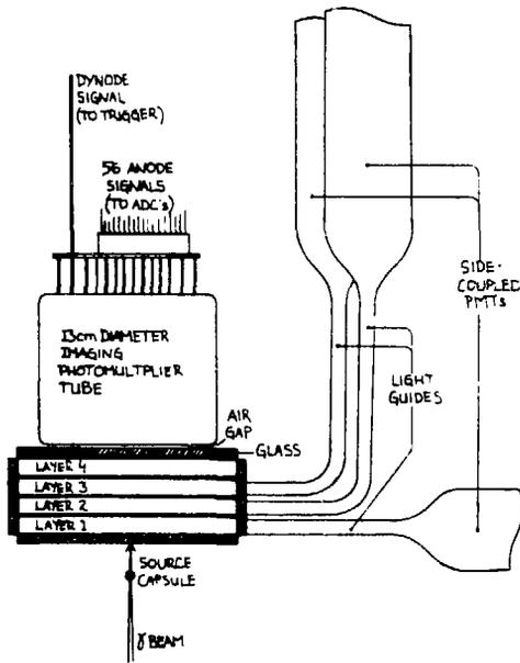
Fig. 1. Apparatus used for testing the layered scintillator
