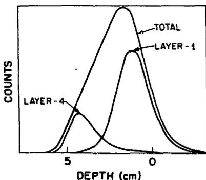
Fig. 4. Number of events as a function of depth estimated by second moment, of the emitted light distribution for all events (total), those interacting in layer-1, and those in layer-4
