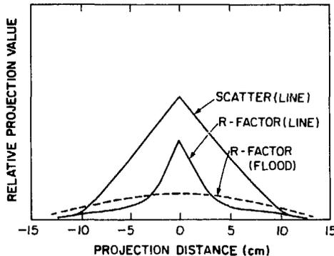
Fig. 6. Simulated scattered radiation projection from a line source in a 20 cm water cylinder (upper solid curve), its ratio to pin-sink identified scattered radiation (lower solid curve), and a similar ratio for a 20 cm flood source (dashed curve)
