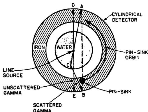
Fig. 5. Conceptual design of a pin-sink apparatus for sampling scattered radiation during PET emission scanning
