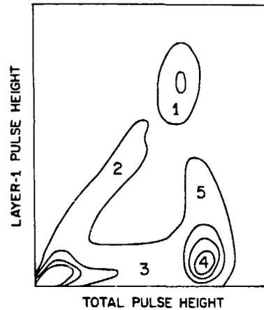
Fig. 2. Contour plot of the number of events as a function of the pulse height in the imaging PMT (horizontal) and the pulse height in the side-coupled PMT attached to layer-1 of the layered scintillator (vertical)
