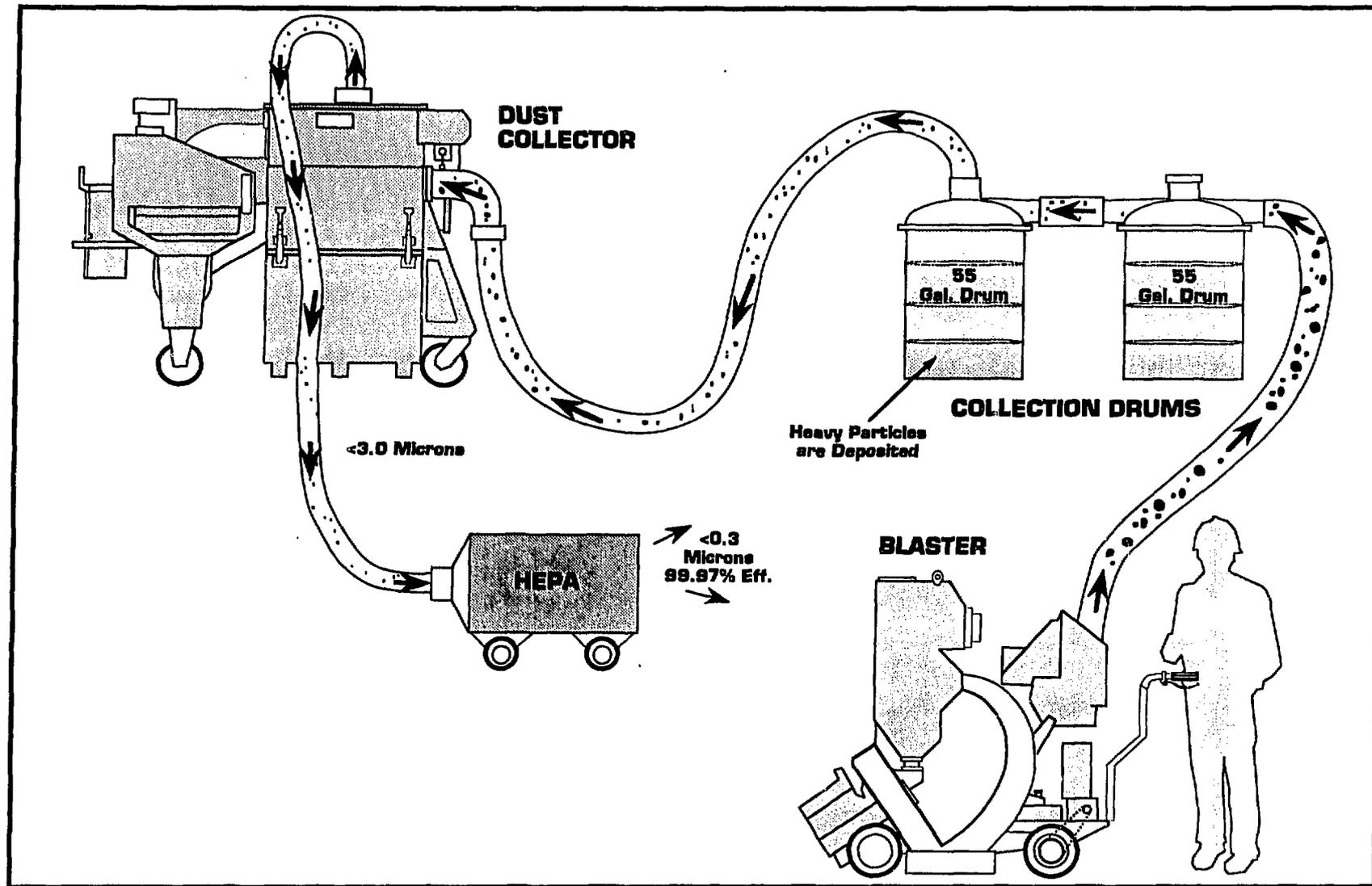
Fig. 3. Shot blast cleaning system.
