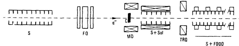
Fig. 10 Electron generated positron source
