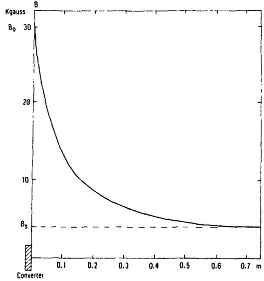
Fig. 16 Field profile of the adiabatic device
