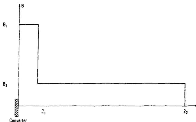
Fig. 13 Field profile of the quarter wave transformer
