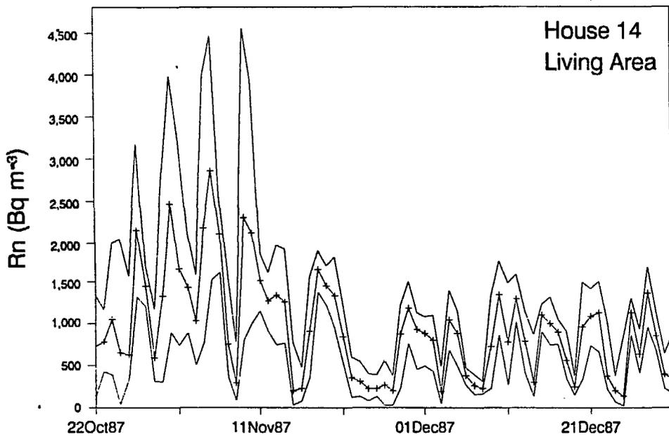
Fig. 1. Measurements of  $^{222}\text{Rn}$  during fall in two Huntsville houses; the upper and lower curves represent daily maximum 30-minute integrated measurement while the middle curve shows the daily average  $^{222}\text{Rn}$  concentration.
