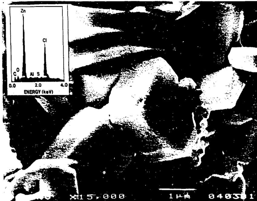
**Fig. 1** Zinc chloride crystal present in INEL incinerator fly ash magnified 15,000 times by scanning electron microscope and associated energy dispersive x-ray spectrum.
