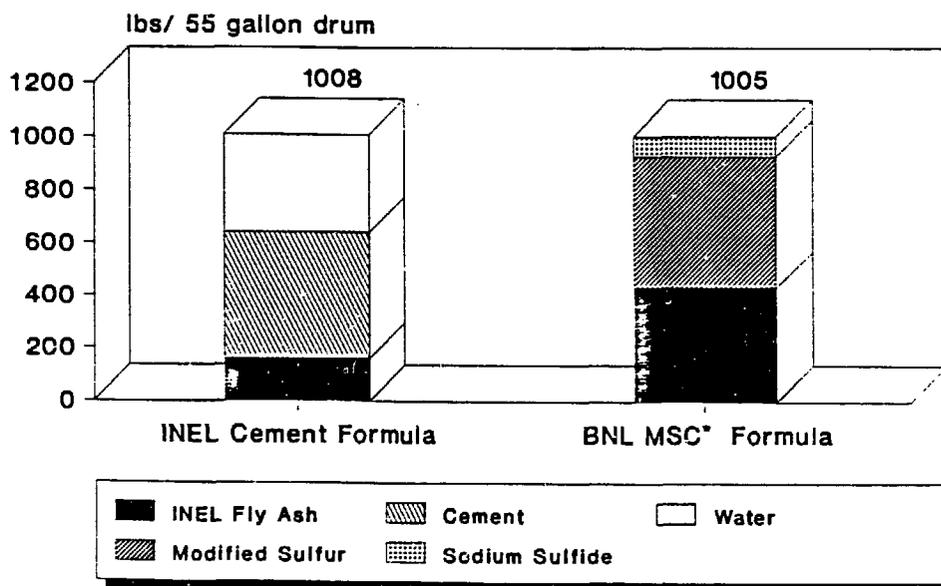
Fig. 4 Comparison of waste loadings for encapsulation of INEL incinerator fly ash in modified sulfur cement and portland cement. (\*MSC = Modified Sulfur Cement.)
