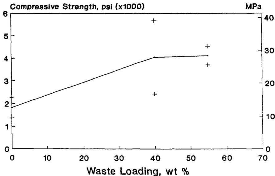
Fig. 3 Compressive strength data for INEL incinerator fly ash encapsulated in modified sulfur cement. (Data shown are mean values for 3 replicates (5 for 55% samples); with error bars at 95% confidence interval.)
