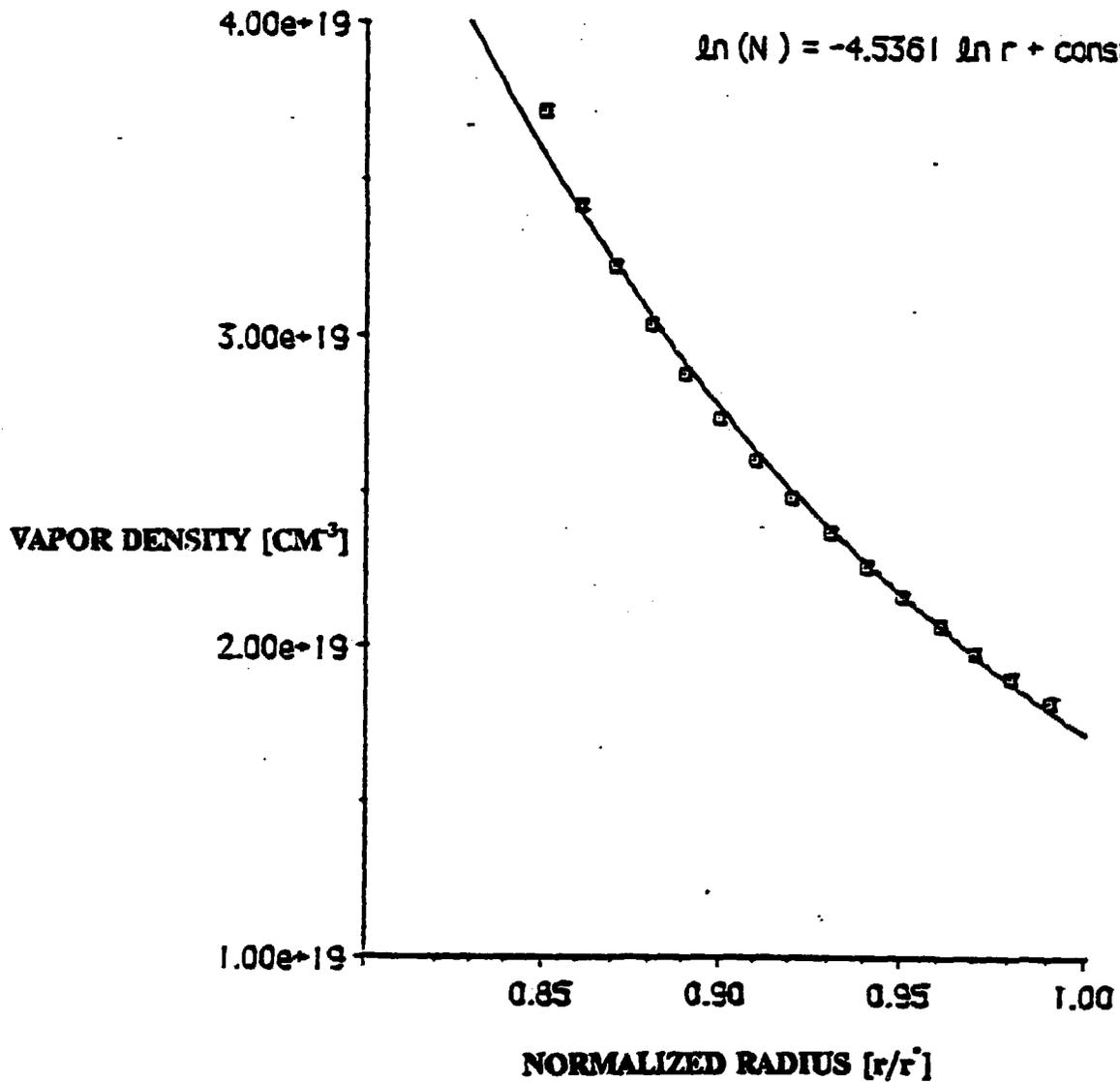
Figure 1. Scaling of the vapor density with normalized radius inside the singular surface (normalized to the singular surface) for the self-consistent solution.
