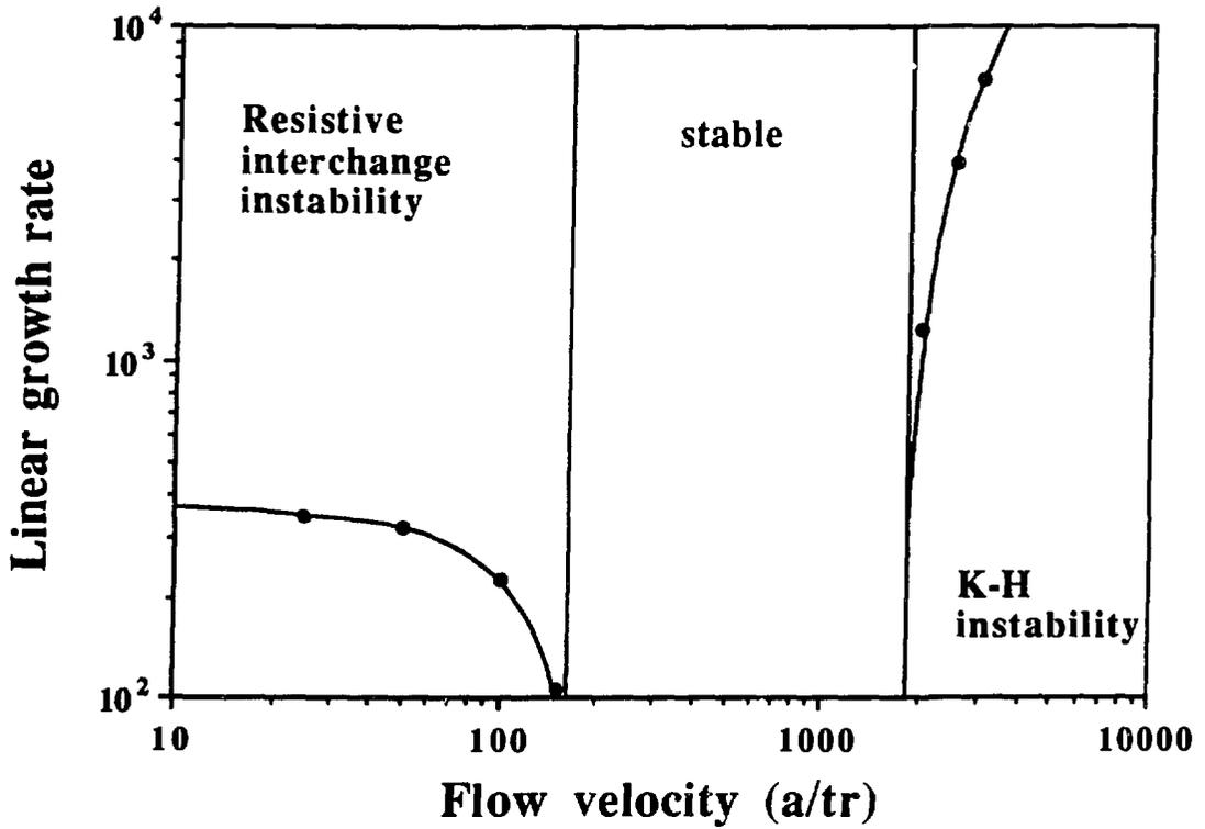
Fig. 1. Linear growth rate of the  $m = 3$  mode as a function of the equilibrium poloidal flow velocity.
