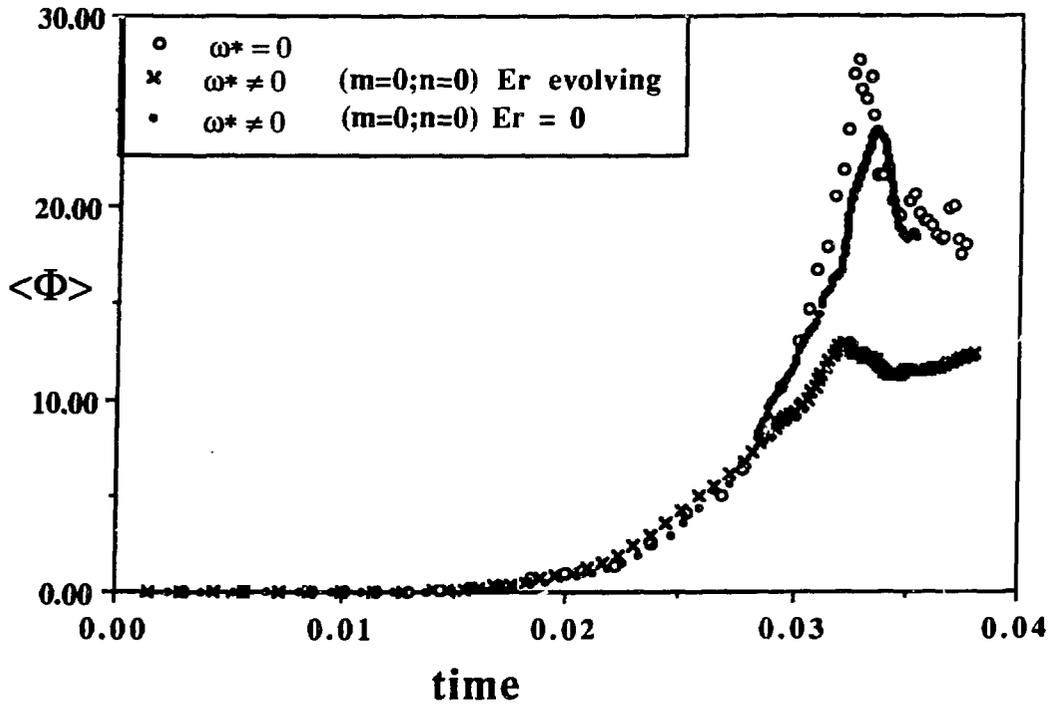
Fig. 3. Evolution of the electrostatic potential fluctuations with and without diamagnetic effects. In the later case, the stabilizing effects of the self-generated electric field are made evident by comparing with a case where the electric field is forced to be zero.
