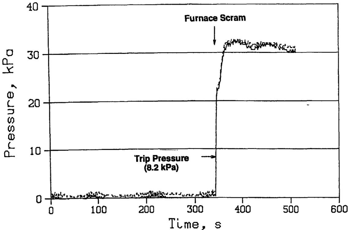
Fig. 4. Pressure transducer responses in a pressurized capsule test with a fusible seal.
