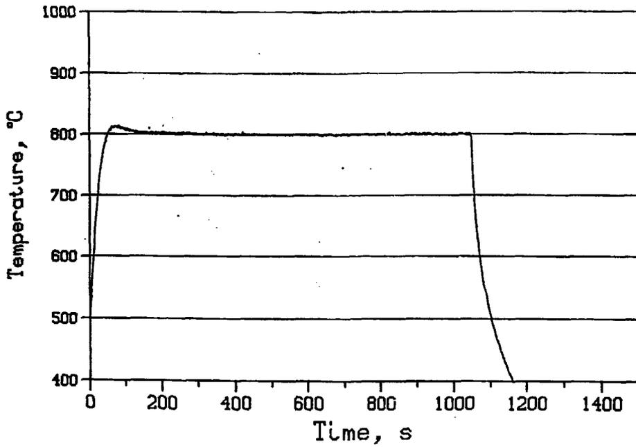
Fig. 2. Typical time-temperature history of the computer-controlled WPF system.
