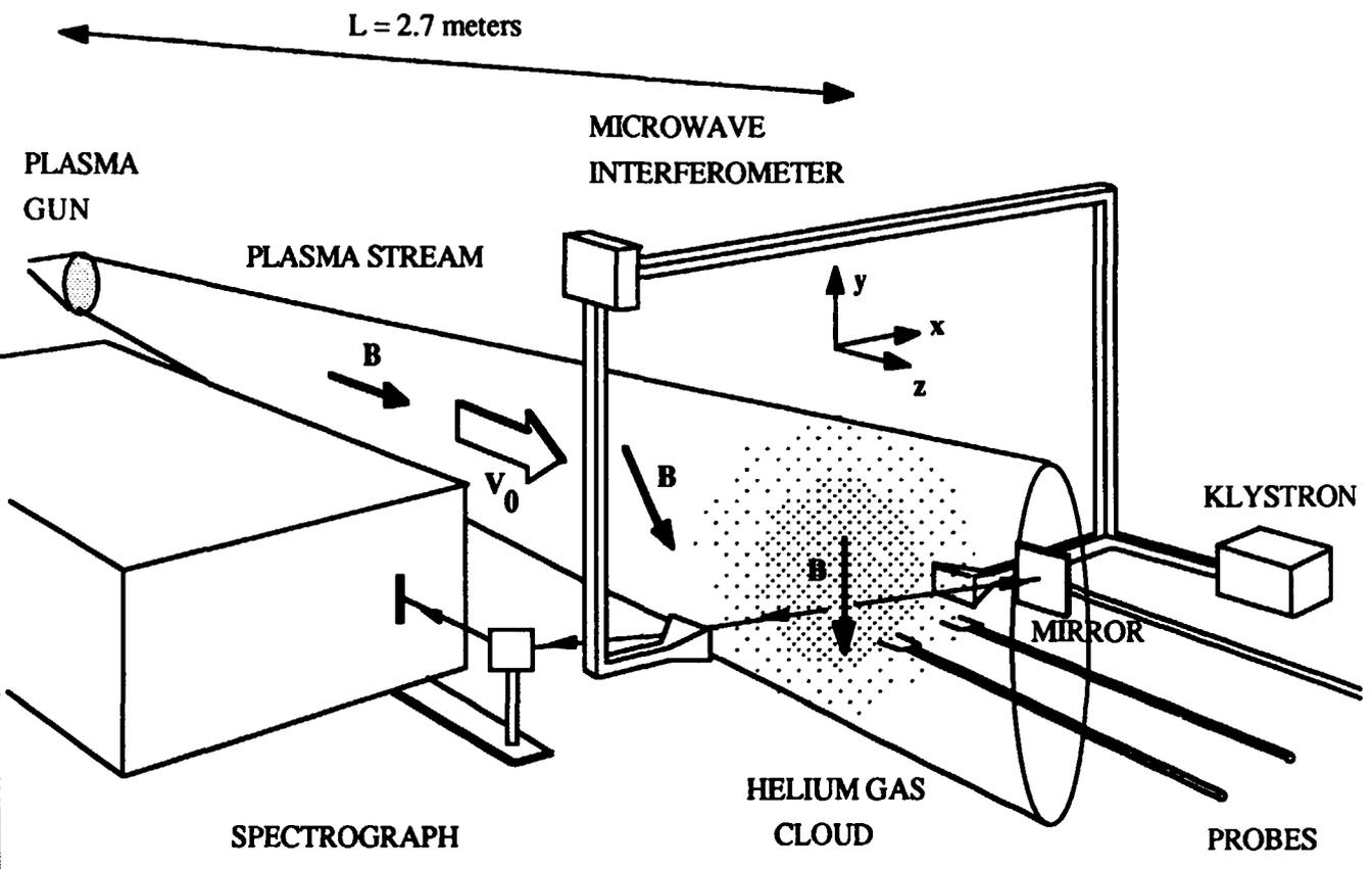
Fig. 3. The plasma source and the diagnostics equipment.
