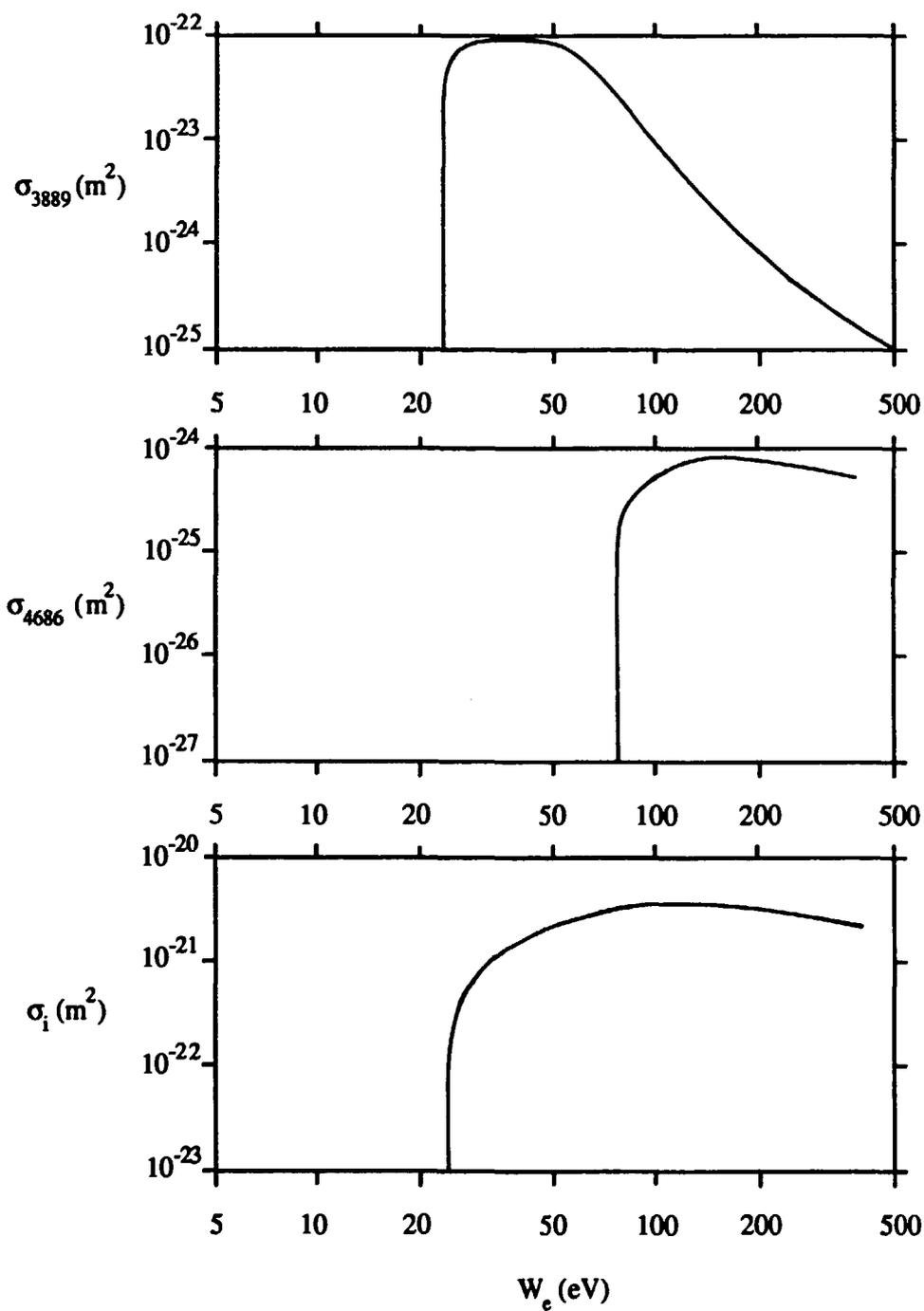
Fig. 5. Cross sections for electron impact excitation of the He I line 3889 Å, and the He II line 4686 Å, both from the ground state of He I, and for electron impact ionization.
