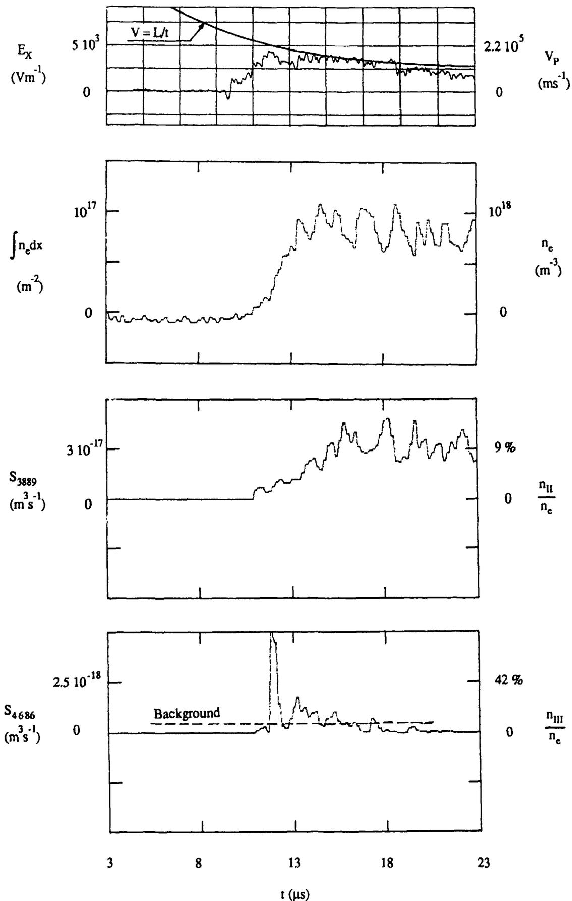
Fig. 7. Measurements for low column helium density. The scales to the left denote measured quantities, and the scales to the right calculated quantities. The relative populations  $n_{II}/n_e$  and  $n_{III}/n_e$  are derived from Eq. 4 and 5. For  $n_{II}/n_e$ , the scale is only accurate before 13 ms; for later times, the experimental curve is an upper limit to the real  $n_{II}/n_e$ .
