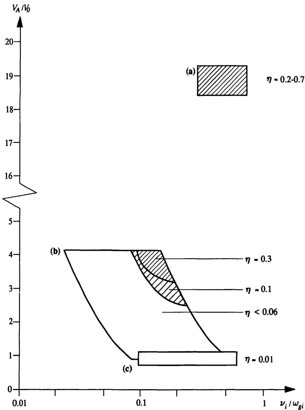
Fig. 12. The  $\eta$  value as function of  $V_A/V_0$  and  $\nu_i/\omega_{gi}$ : (a): The experiments by Danielsson, 1972, and Danielsson and Brenning, 1975. (b): The present experiments. (c): The experiments by Brenning, 1981b.
