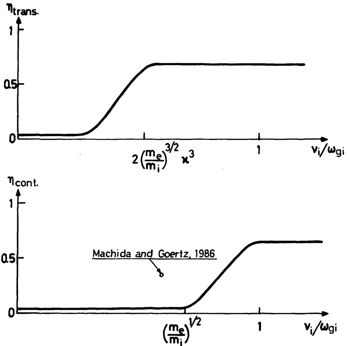
Fig. 2. The variation of the energy transfer efficiency  $\eta$  with  $v_i/\omega_{gi}$  (from Axnäs and Brenning, 1988). The upper graph shows the initial state of a transient situation, and the lower shows a homogeneous steady state situation (drawn schematically after Galeev, 1981). The circle in the lower graph shows the result of a computer simulation for a case in between transient and steady state.
