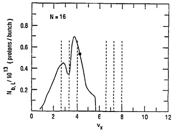
Fig. 5 Intrinsic space charge limit versus  $\nu_x$  for the PS booster at different distances from the diagonal  $\nu_x = \nu_y$ .
