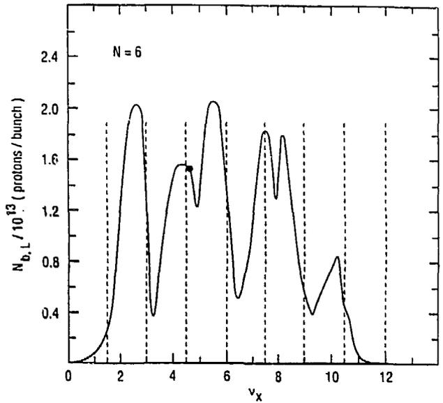
Fig. 4 Intrinsic space charge limit versus  $\nu_x$  for the PS booster.  $\nu_y = \nu_x + 1.35$ .
