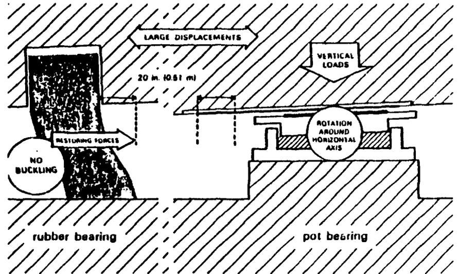
Fig. 4. Alexisismon Sliding Pot Bearings System
