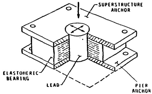
Fig. 2. Laminated Elastomeric Bearings with Lead Plug
