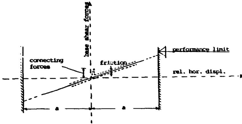
Fig. 6. Linear Isolation System
