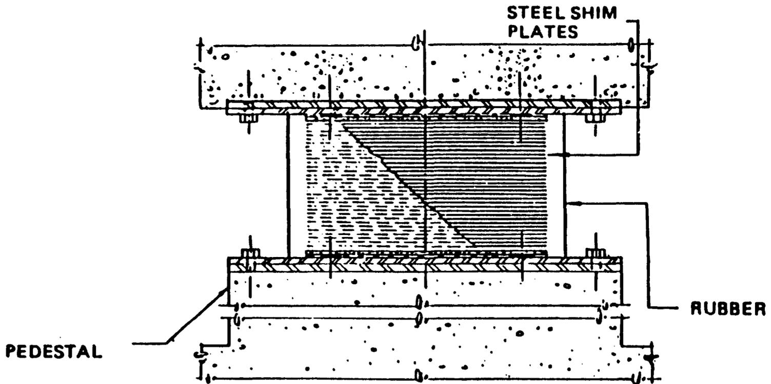
Fig. 1. Laminated Elastomeric Bearings
