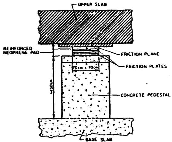
Fig. 3. Combined Laminated elastomeric Bearing and Sliding Plates
