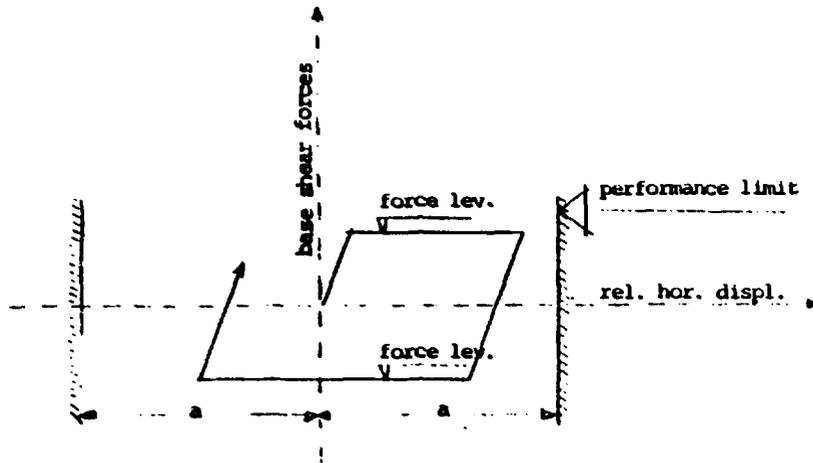
Fig. 7. Bilinear Isolation System
