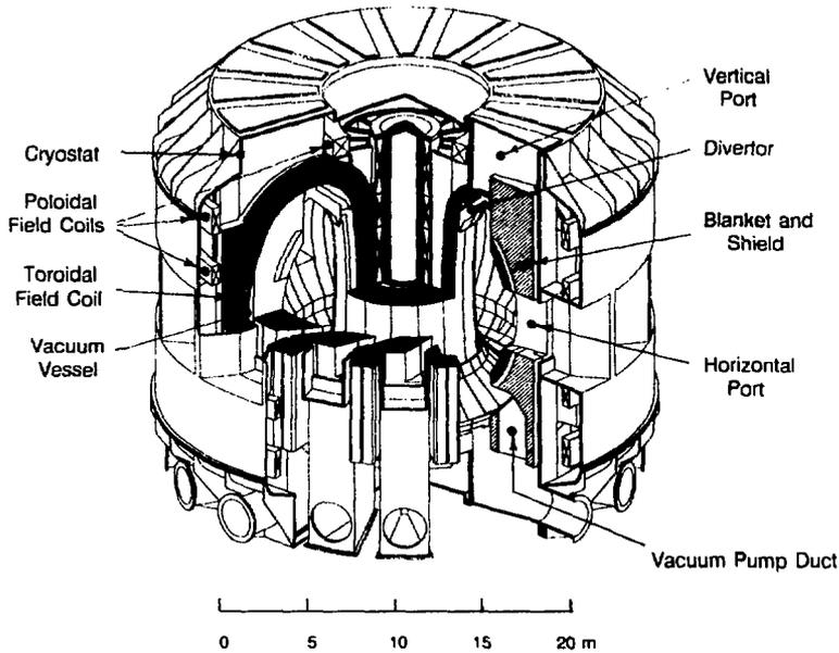
Fig. 2. Basic Elements of ITER Tokamak
