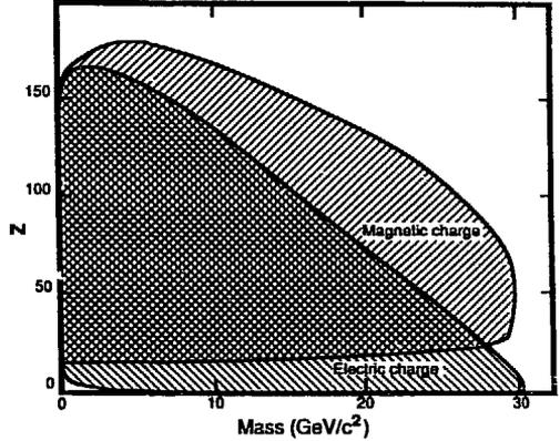
Figure 2. Mass-charge combinations to which CR-39 detector has finite sensitivity. Regions sensitive to electric and magnetic charges are indicated separately.
