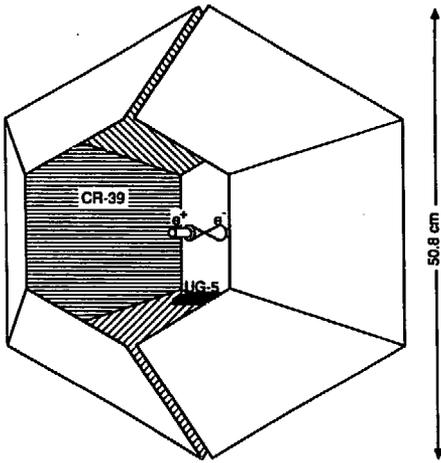
Figure 1. Configuration of Nikko-Maru detector, showing halves of CR-39 slightly separated. The UG-5 is inside the vacuum while the CR-39 is outside.
