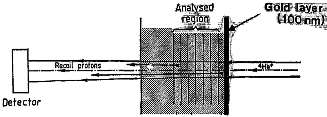
**Fig. 1.** : Elastic recoil detection in transmission mode
