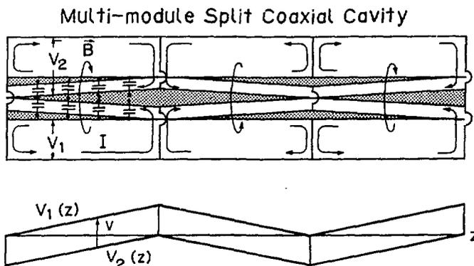
Fig. 4. Conceptual diagram of a multi-module split coaxial cavity resonator.
