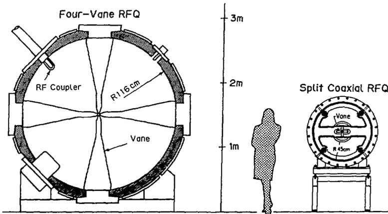
Fig. 2. Comparison between the sizes of 25.5-MHz RFQ's: the JHP SCRFAQ and a four-vane RFQ.
