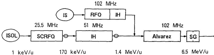
Fig. 1. System structure of the JHP heavy ion linac.
