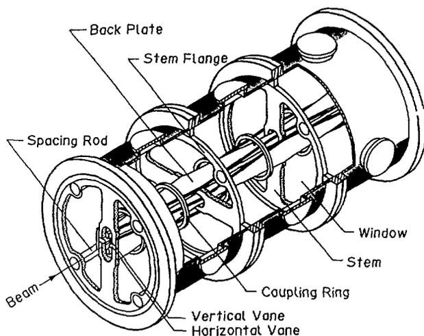
Fig. 6. Structure of the 25.5-MHz prototype model.
