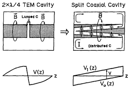
Fig. 3. Principle of a split coaxial resonator.
