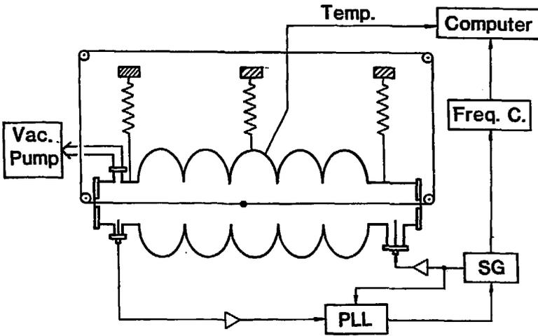
Fig.4 Configuration of bead-perturbation measurement system.
