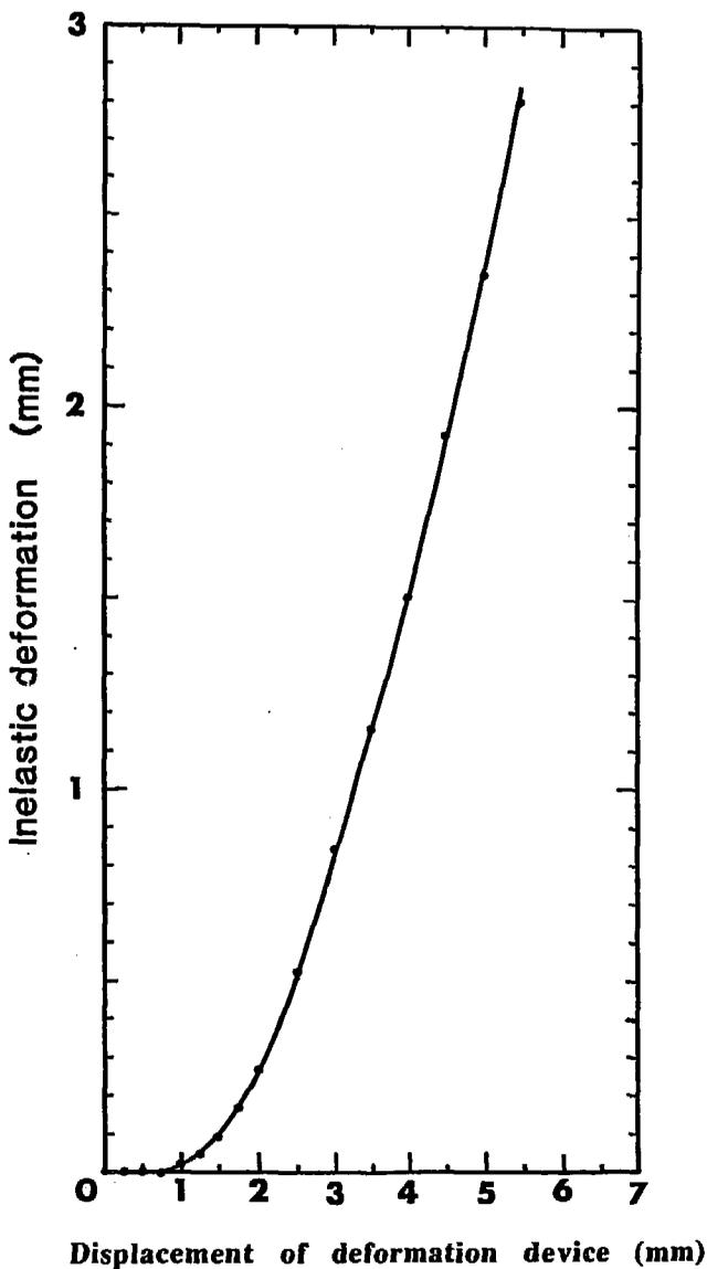
Fig.12 Inelastic deformation ( squeezed ) as a function of the displacement of the deformation device.
