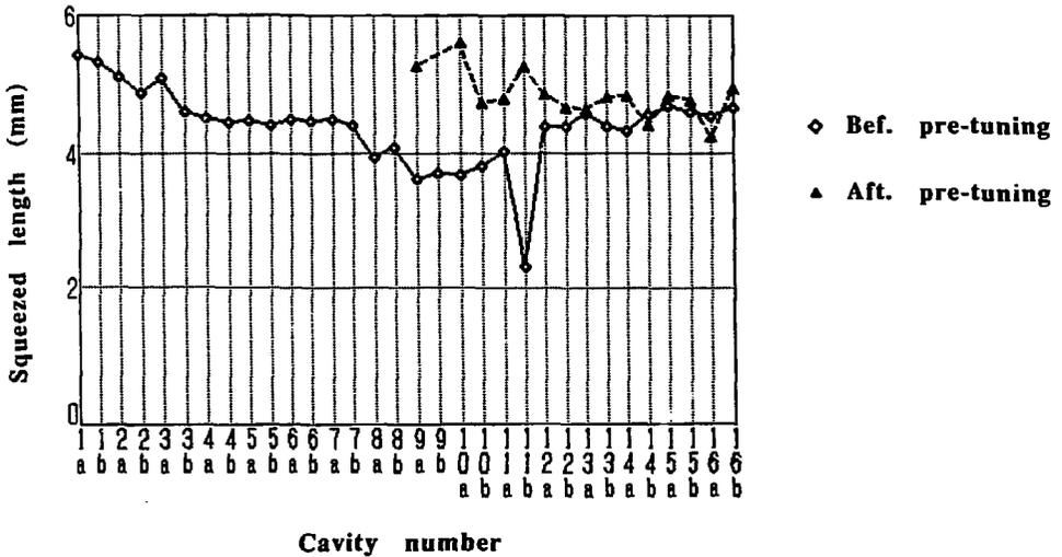
Fig.10 Squeezed length of the cavity by evacuation before and after pre-tuning.
