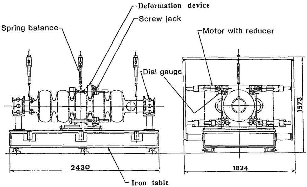
Fig.2 Pre-tuning instrument.
