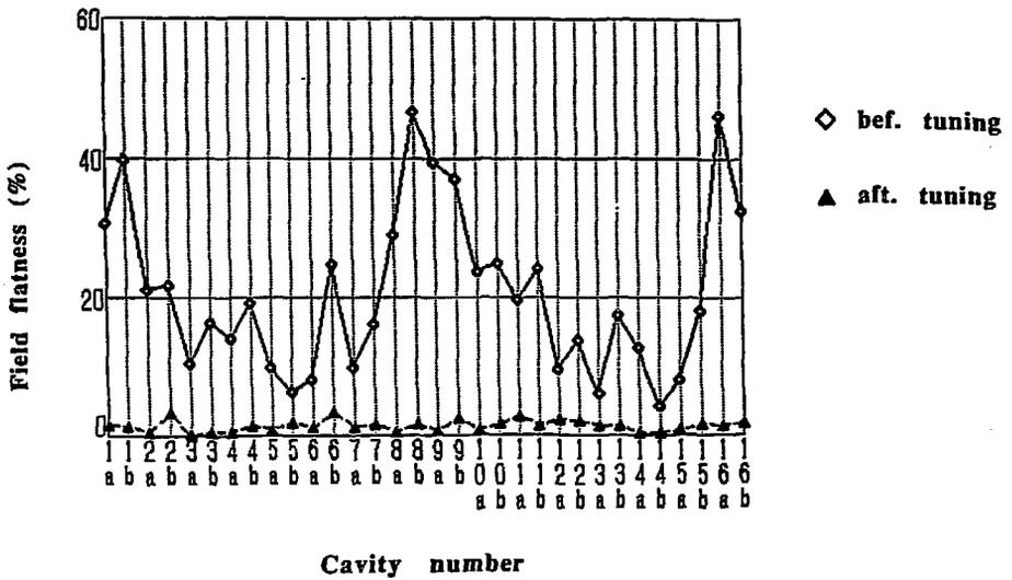
Fig.8 Field flatness of the cavities before and after pre-tuning.
