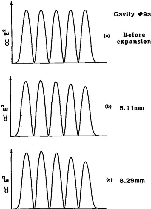
Fig.16 An example of the change of field flatness during the expansion test.
