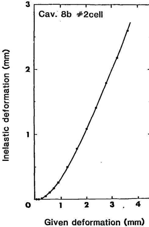
Fig.14 Inelastic deformation as a function of the given deformation.
