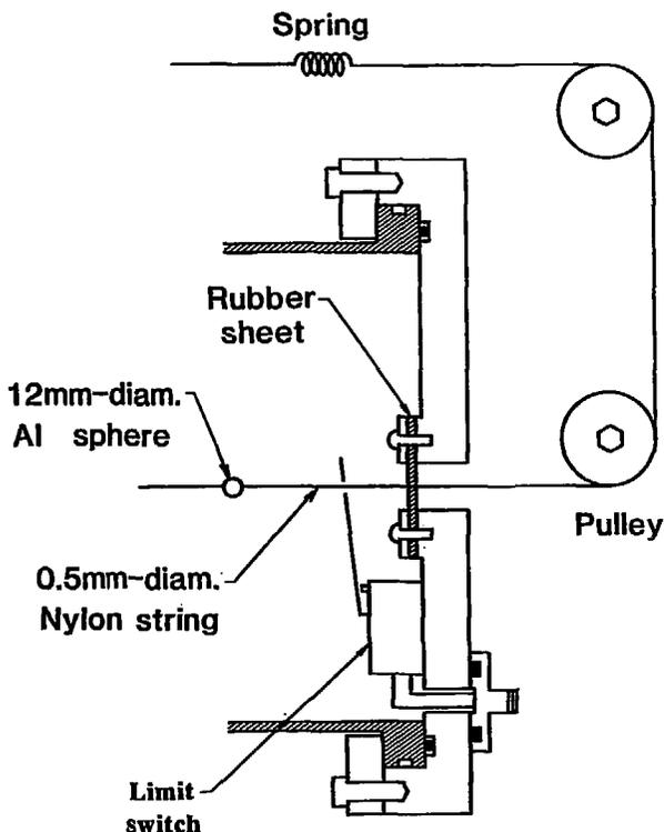
Fig.3 Cross-sectional view of the end beam-tube flange.
