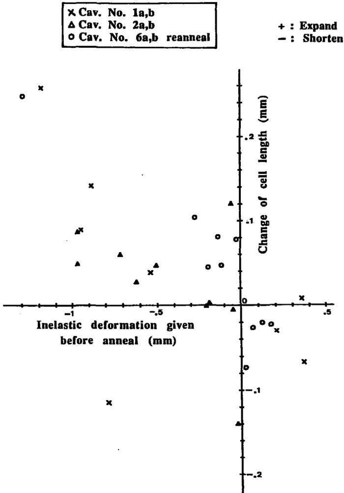
Fig.9 Changes of the cell lengths after the annealing of the pre-tuned cavities as a function of the given inelastic deformation lengths.
