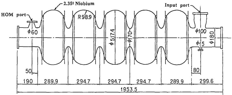
Fig.1 Photo of TRISTAN superconducting cavity and its nominal dimension.
