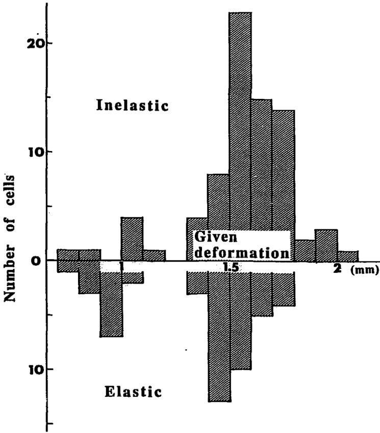
Fig.17 Number of the cells deformed elastically or inelastically in expansion test as a function of the deformation given to each cell.
