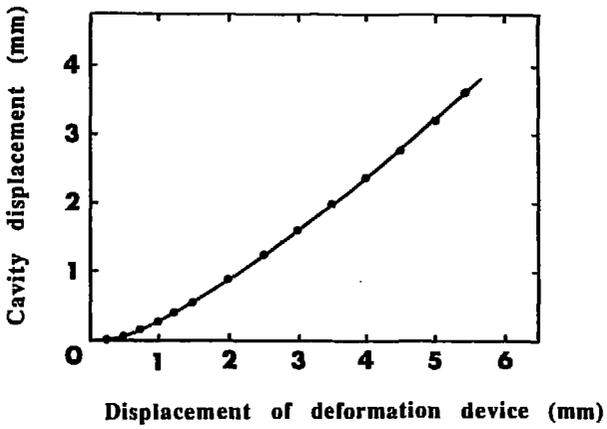
Fig.13 Cavity displacement as a function of the displacement of the deformation device.
