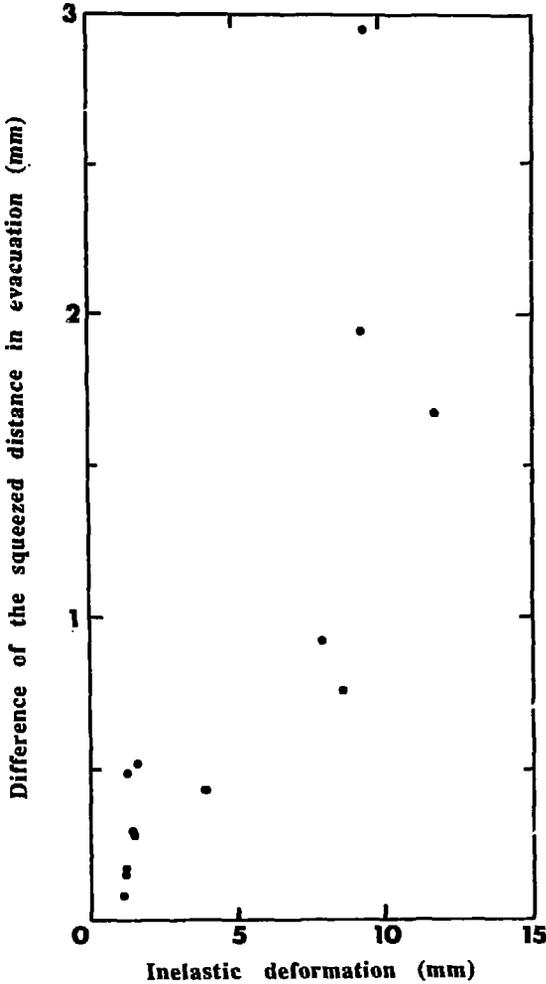
Fig.11 Difference of the squeezed distance in evacuation between before and after pre-tuning as a function of the total inelastic deformation length of each cavity.
