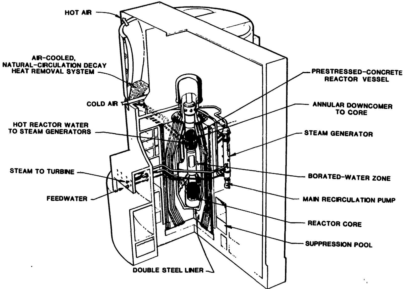
Fig. A.2. Proposed PIUS design by ABB Atom.
