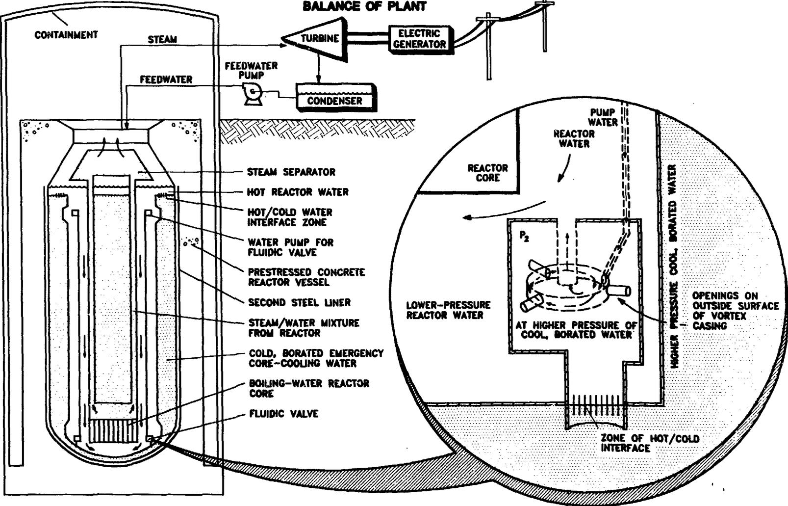
Fig. A.3. Process Inherent Ultimate Safety Boiling-Water Reactor.
