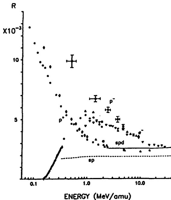
Fig. 2. The ratio  $R$  between double and single ionization cross sections for antiprotons, protons, and electrons in He. The broken and full curves labelled  $sp$  and  $spd$  are first Born results of Ford and Reading, Ref. 4, item 2. Filled squares, antiproton data from Ref. 3. Other filled symbols, electron data. Open symbols, proton data. References to experimental data are given in Ref. 4, item 2.
