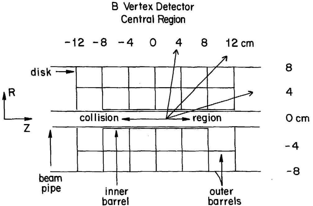
Figure 3: The SSC B Vertex Detector Central Region.
