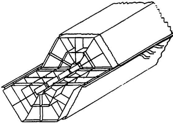
Figure 4: The Vertex Detector Model built by Hans Jostlein of Fermilab. This is being used to study heat dissipation and alignment issues.
