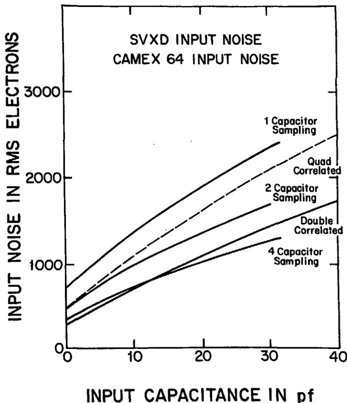
Figure 7: The Noise versus Input Capacitance for the SVXD chip and the CAMEX chip. The different modes of operation are shown. This data courtesy R. Yarema of Fermilab.
