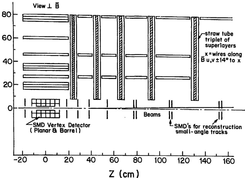
Figure 8: View of the BCD straw tracker showing box-like structure. There are roughly 250,000 4mm diameter straws in this design. Also shown are the silicon vertex detectors.
