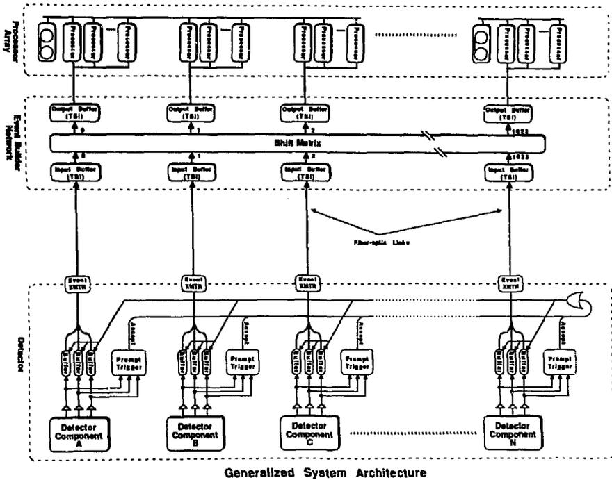
Figure 9: Generalised System Architecture is shown. The data flows upward. The dashed line indicates electronics mounted directly on the detector. The data is transmitted from the detector to the event builder switch after a trigger decision via fiber optic links. The event builder passes the data to a processor farm with a serial link.
