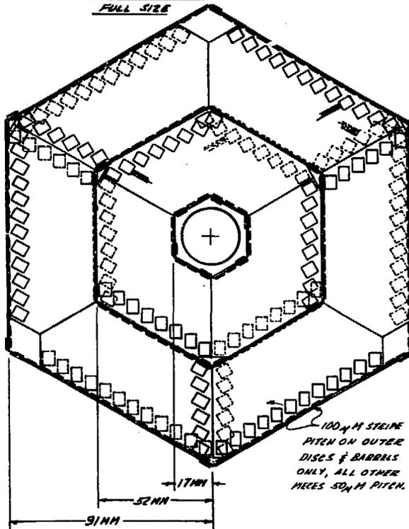
Figure 6: Fermilab BCD Silicon Vertex Detector Central Station. The view is in the x-y plane. Three barrels can be seen in projection and inner and outer disks are shown with the chips mounted. Solid boxes are amplifiers on near side and dashed boxes are amplifiers on the underside. Beam pipe is shown as a circle and lines represent strips.
