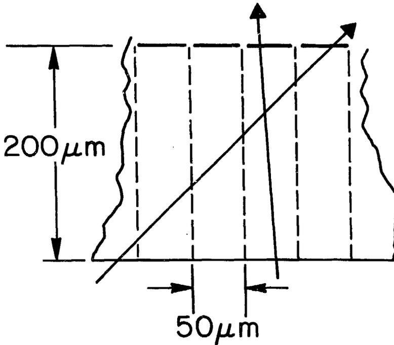
Figure 5: Tracks at incident at  $45^\circ$  deposit  $< 6000$  electron/hole pairs. Observation of this small signal requires very low noise amplifiers.
