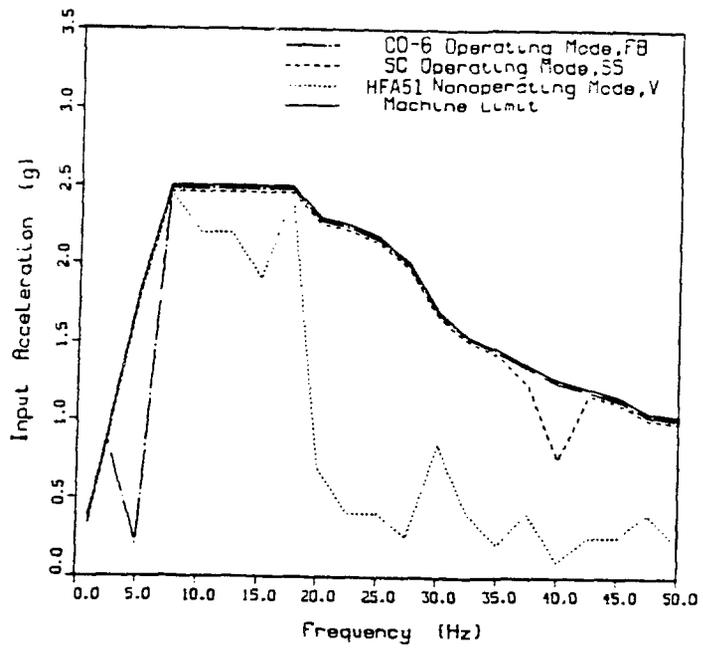
Figure 1 Influence of Vibration Frequency Sine Dwell Capacity Level
