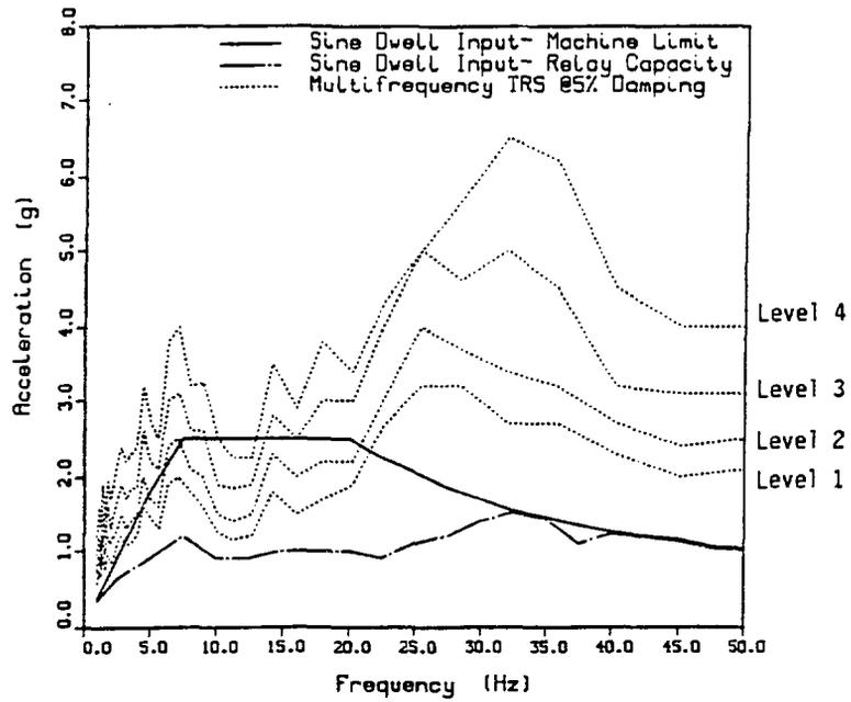
Figure 12 Generation of Capacity TRS
