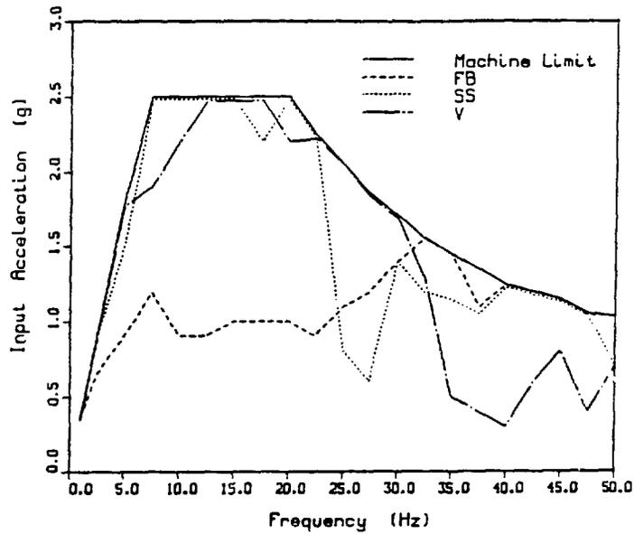
Figure 2 Sine Dwell Capacity Level SG, Specimen 3 Nonoperating Mode, NC Contact
