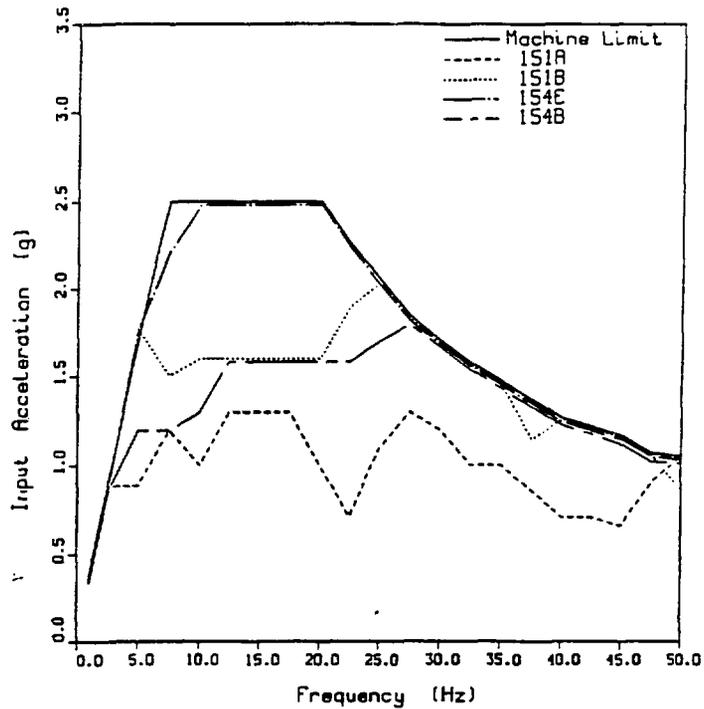
Figure 14 Dynamic Similarity of HFA Relays Sine Dwell Capacity Level FB Direction, Nonoperating Mode, NC Contact
