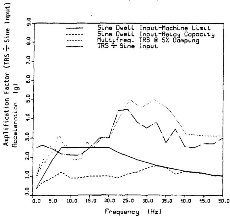
Figure 13 Correlation of Sine Dwell Input and Multifrequency TRS, SG, Specimen 3 FB Direction, Nonoperating Mode, NC Contact
