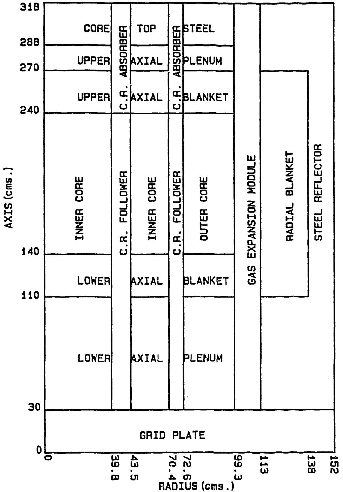
Fig.2 Cylindrical Geometry Model of PFBR Core
