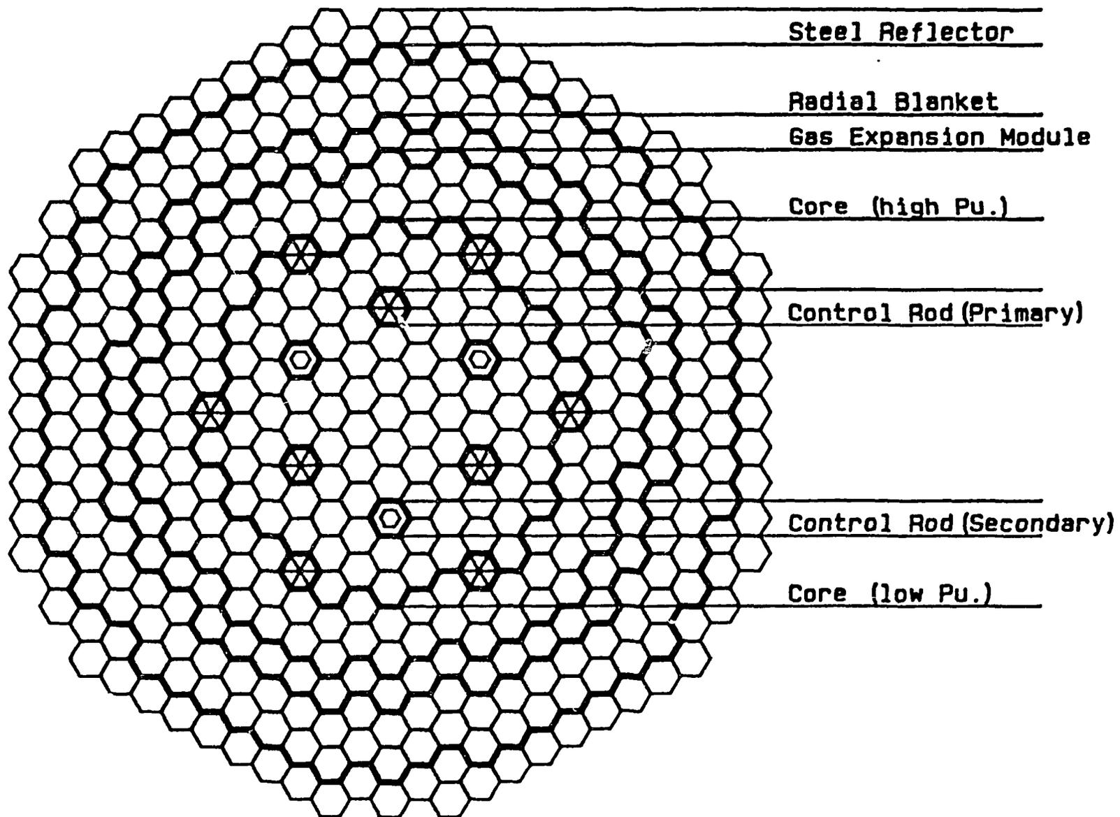
Fig. 1 PFBR Core Configuration
