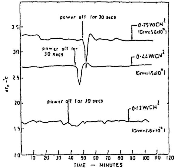
FIG. 8. Stability test at different heat fluxes (without throughflow).
