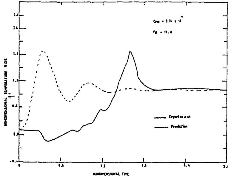
FIG. 4. Transient behaviour at  $Fr > 1$ .
