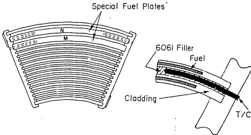
Fig. 4. Double Plate Fuel Element for Core-I Tests
