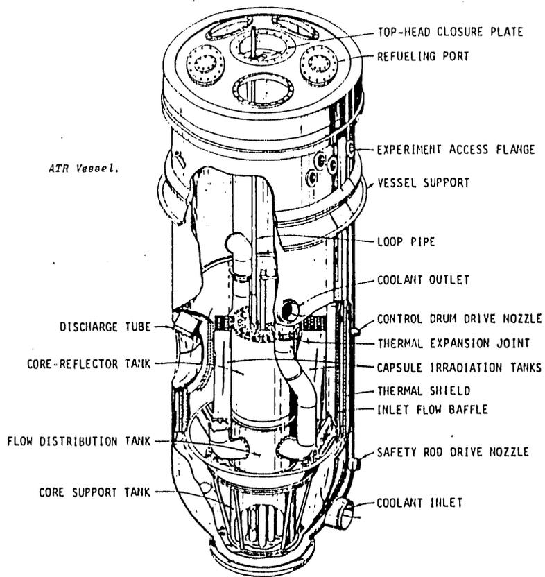
Fig. 1. ATR Reactor Vessel
