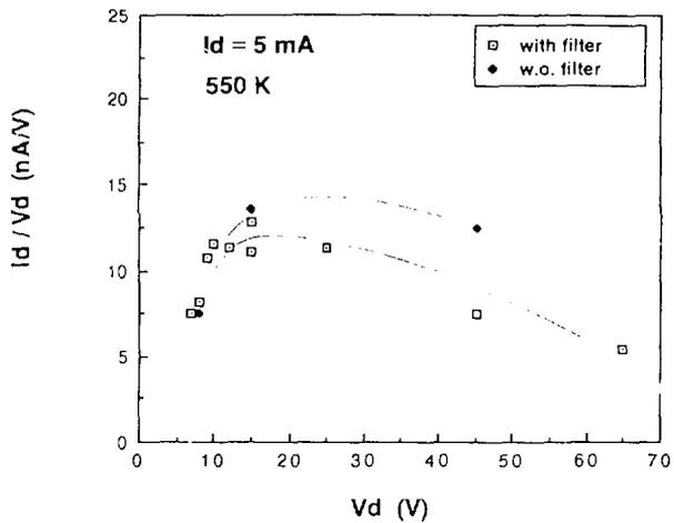
Fig. 6 The normalized  $\text{Na}^-$  current ( $I^-$ ) by the discharge voltage ( $V_d$ ) as a function of  $V_d$ . Open circles indicate those with the magnetic filter and closed without it.
