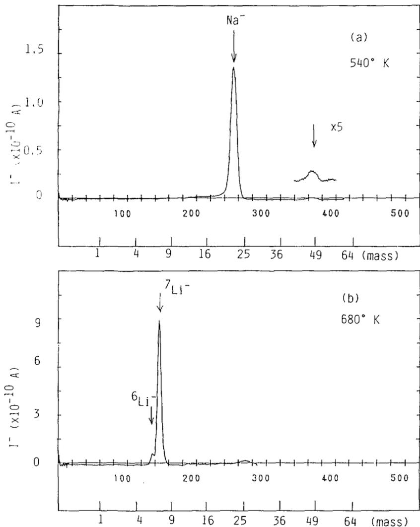
Fig. 2. Momentum spectra of  $\text{Na}^-$  (a) and of  ${}^6\text{Li}^-$  and  ${}^7\text{Li}^-$  (b). In Fig (a), a small peak of mass number = 46 is seen, indicating a possible existence of  $\text{Na}_2^-$ .
