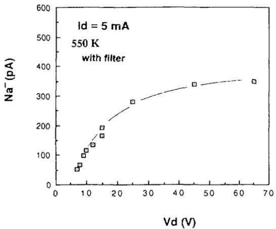
Fig. 4 The dependence of the Na<sup>-</sup> beam current on the discharge voltage measured with the magnetic filter.
