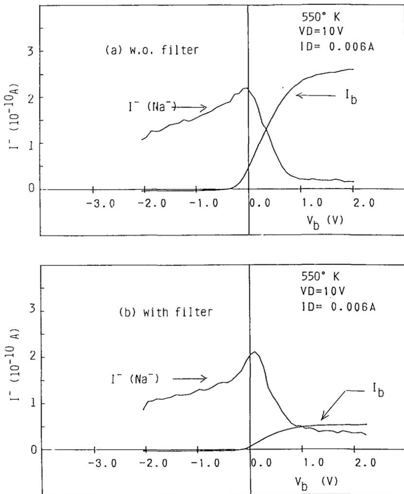
Fig. 5 The dependence on the plasma electrode bias voltage ( $V_b$ ) of the  $\text{Na}^-$  current and the drain current of to the plasma electrode, without the magnetic filter (a) and with it (b).
