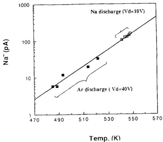
Fig. 3 The heat shield temperature dependence of the  $\text{Na}^-$  beam current .
