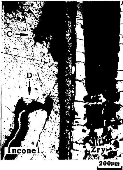
Fig. 15 Interaction between Zircaloy tube and Inconel spacer grid heated at 1573K for 300s in O 2 .
