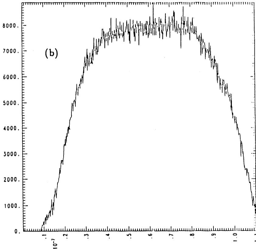
**Figure 1.** (a) Beam current versus time for the ATA injector problem, using leapfrog time advance for the EM field; (b) using damped time advance with  $\theta = 0.8$ .
