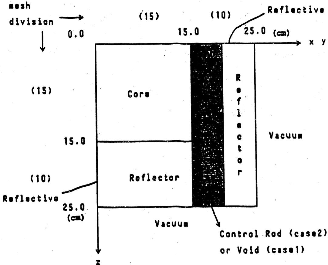
Fig. 1 Calculational model of Model 1 (small LWR)
