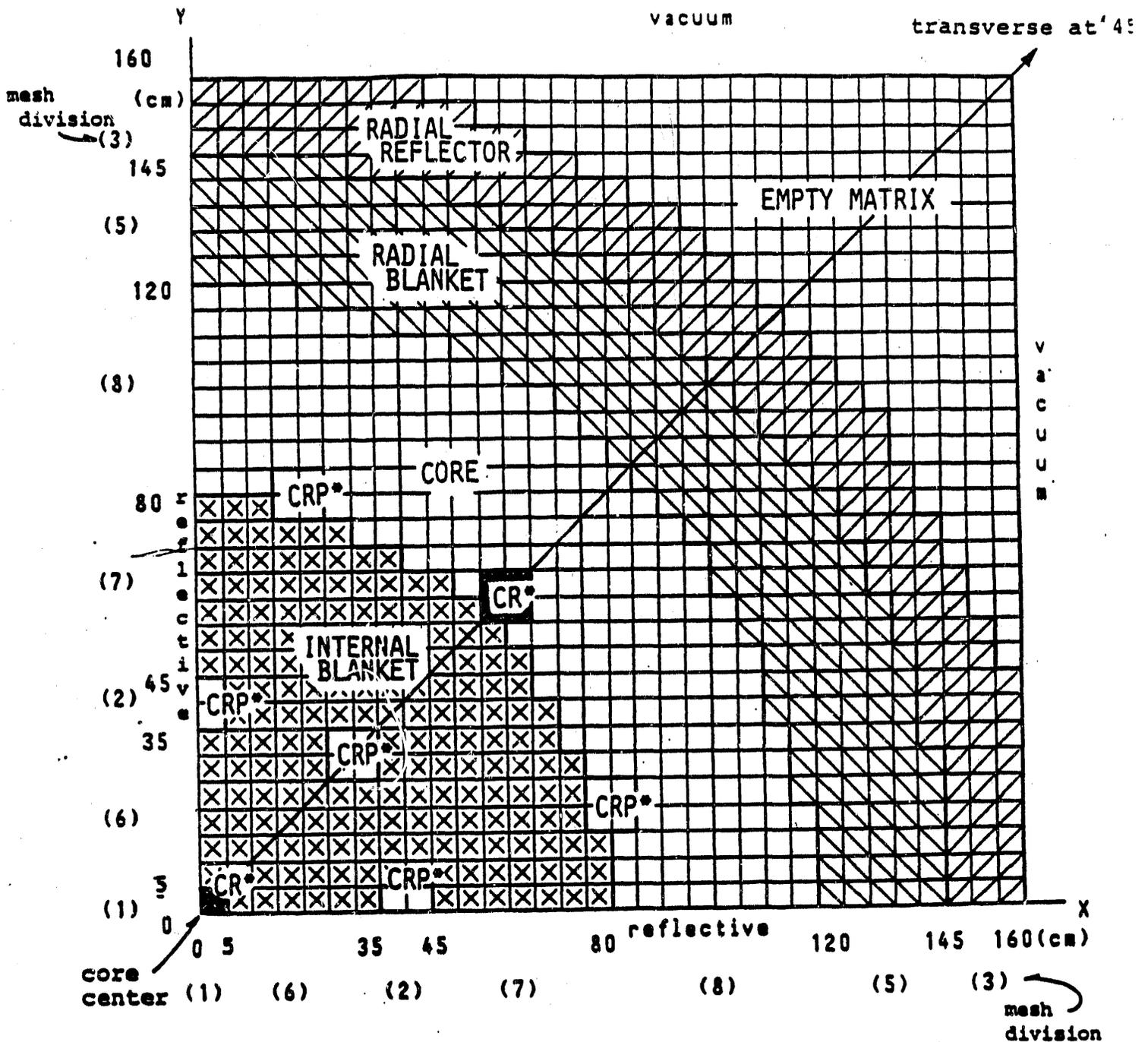
Fig. 3a XY cross sectional view of Model 3, Case 1 & 2 (axially heterogeneous FBR with control rod positions) at core midplane - 32 x 32 mesh, 1/4 core -
