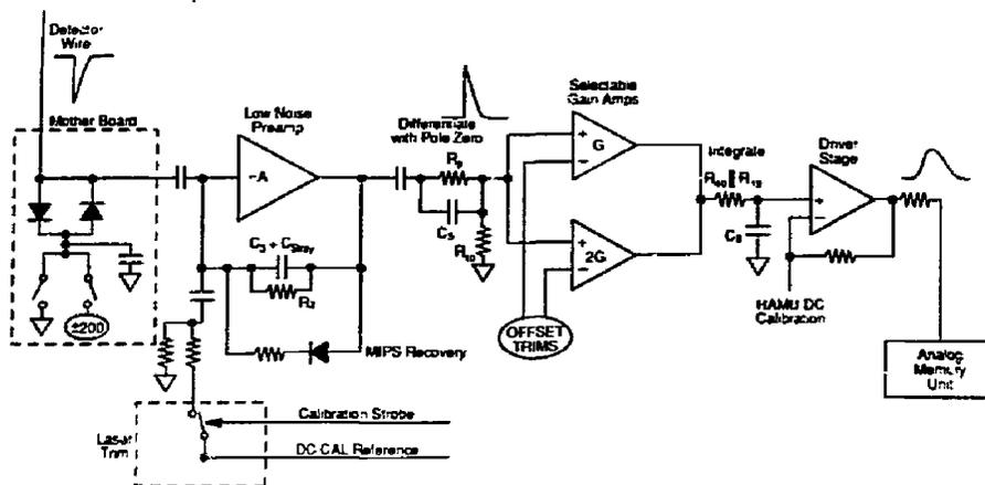
Fig. 1. Block diagram of the front-end system.
