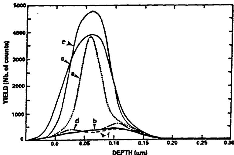
Fig. 3. Mesotaxial growth of a seed sample occurring during reimplantation of  $6 \times 10^{16} \text{ cm}^{-2}$  at  $520^\circ\text{C}$  showing random and aligned RBS spectra respectively from the seed (a,b), after the second implantation (c,d) and after a second anneal at  $800^\circ\text{C}$  (e,f).
