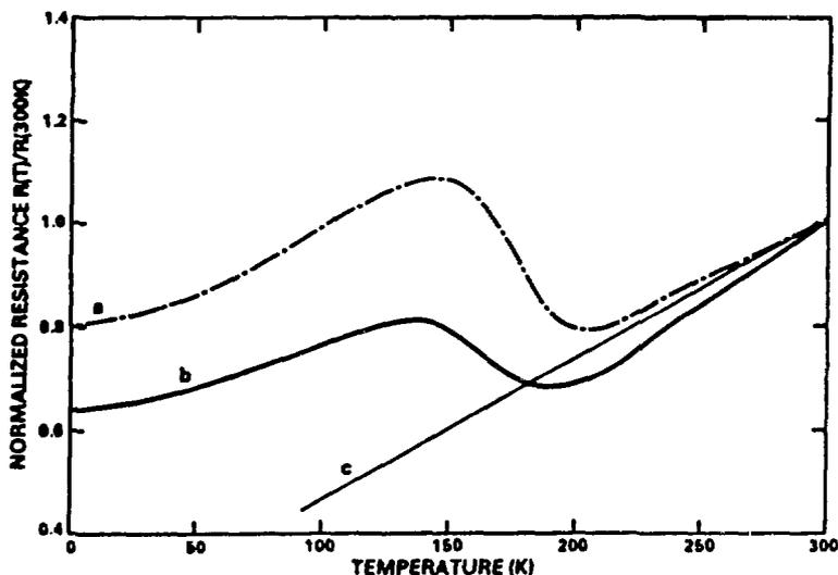
Fig. 4. Normalized resistance versus temperature curves for buried  $\text{ErSi}_2$  layers formed using 170 keV Er ion doses of  $7 \times 10^{16}/\text{cm}^2$  (a) and  $1 \times 10^{16}/\text{cm}^2$  (b). Curve (c) corresponding to the  $\text{ErSi}_2$  layer formed using ultrahigh vacuum codeposition of Er and Si followed by an appropriate thermal annealing [5,6] is shown for comparison.
