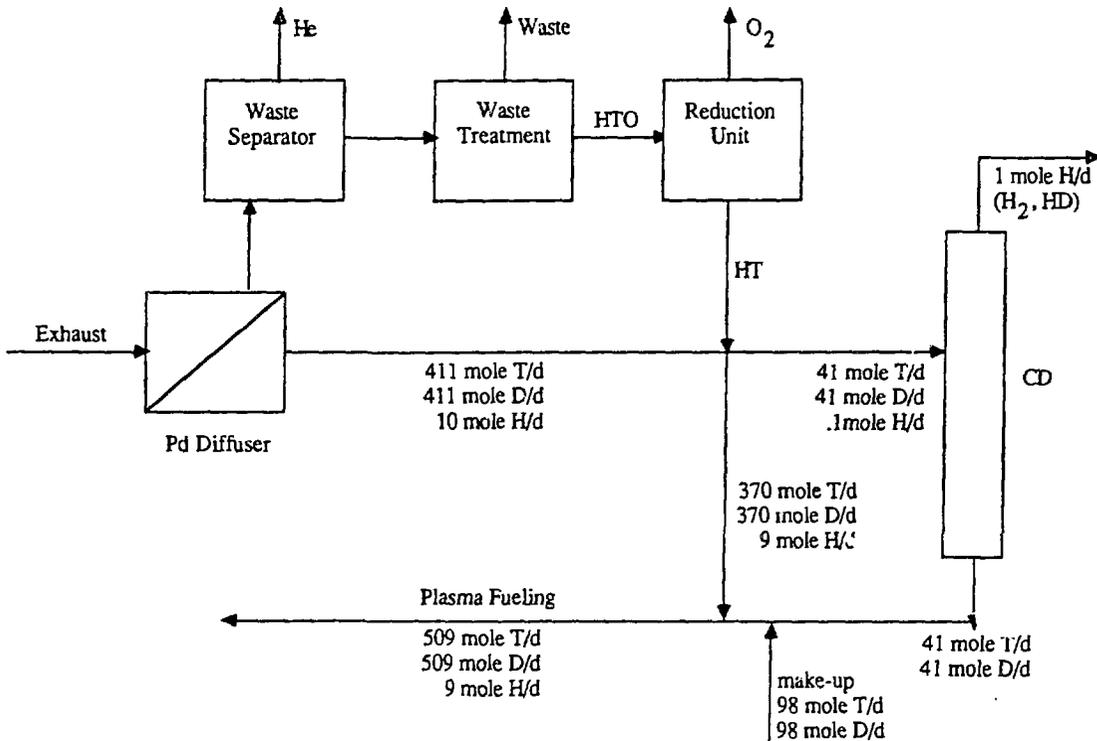
Figure 2. ARIES-I fuel processing flow diagram.
