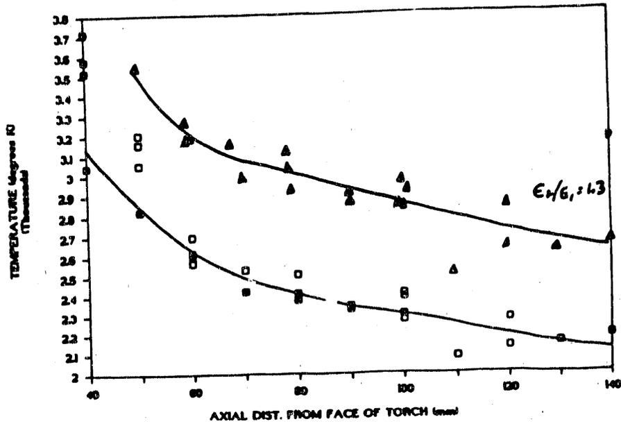
Fig. 5. Average centerline particle temperature data.
