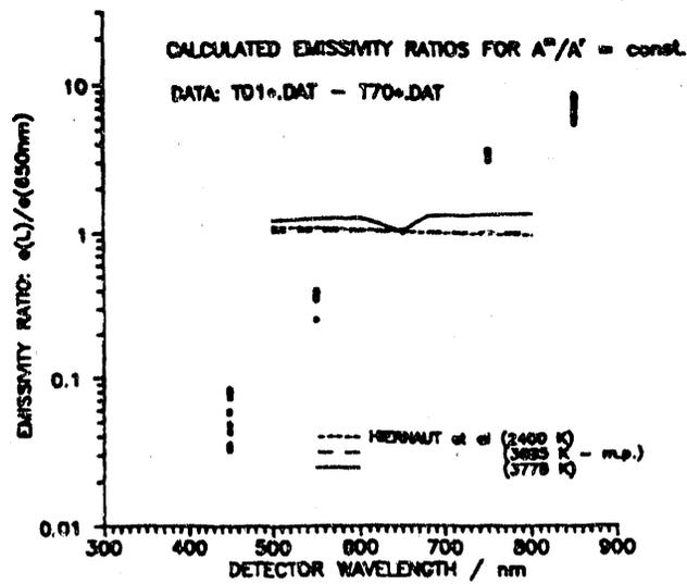
Figure 2. Emissivity ratios at the melting point calculated from radiation signals from pulse-heated tungsten particles.
