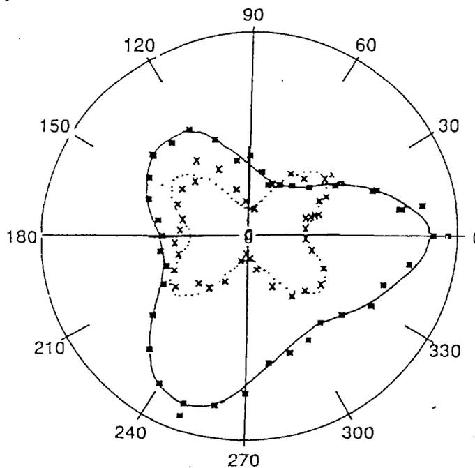
Figure 4. SSHG intensity plotted as a function of rotation of the Fe [110] surface about its normal. The Fe [001] direction is taken as 0°. The dotted curve and the "x" data points is for p polarized incident light and p polarized second harmonic light. This spectra shows the bulk bilateral symmetry of the Fe [110] substrate. The solid curve is for an s polarized incident beam and a p polarized second harmonic signal. Here the three fold symmetry of the FeO [111] surface can be found.
