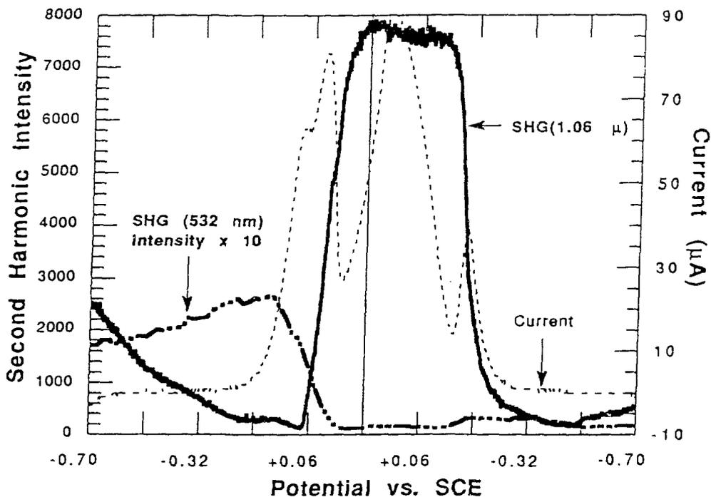
Figure 2. Cyclic voltammogram (CV; light broken line) and second harmonic intensity of a polycrystalline Ni surface. The heavy line is for an incident wavelength of 1.06 μm. The three dot dash heavy line is for an incident wavelength of 532 nm and is 1/10 the intensity of the second SSHG curve.
