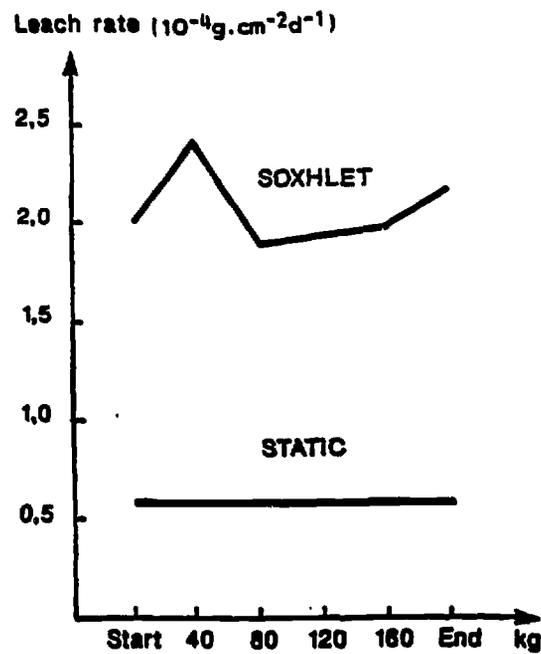
Fig. 7 : Modification of the leach rate of a non radioactive full scale glass during the pouring
