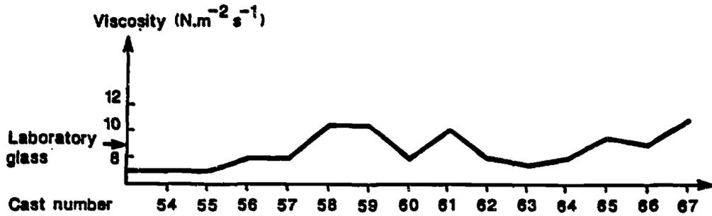
Fig. 4 : Modification of the viscosity versus time (14 consecutive casting operations) of a non radioactive full scale glass
