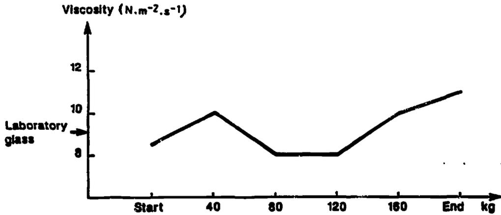
Fig. 5 : Modification of the viscosity of a non radioactive full scale glass during the pouring
