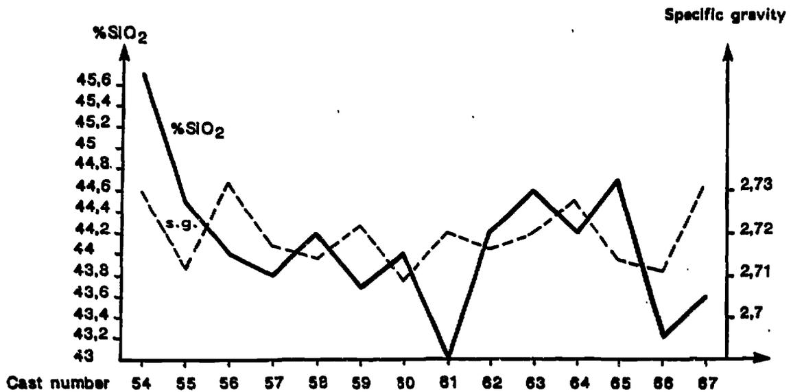
Fig. 2 : Modification of the specific gravity and of the SiO<sub>2</sub> content versus time (14 consecutive casting operations) of a non radioactive full scale glass
