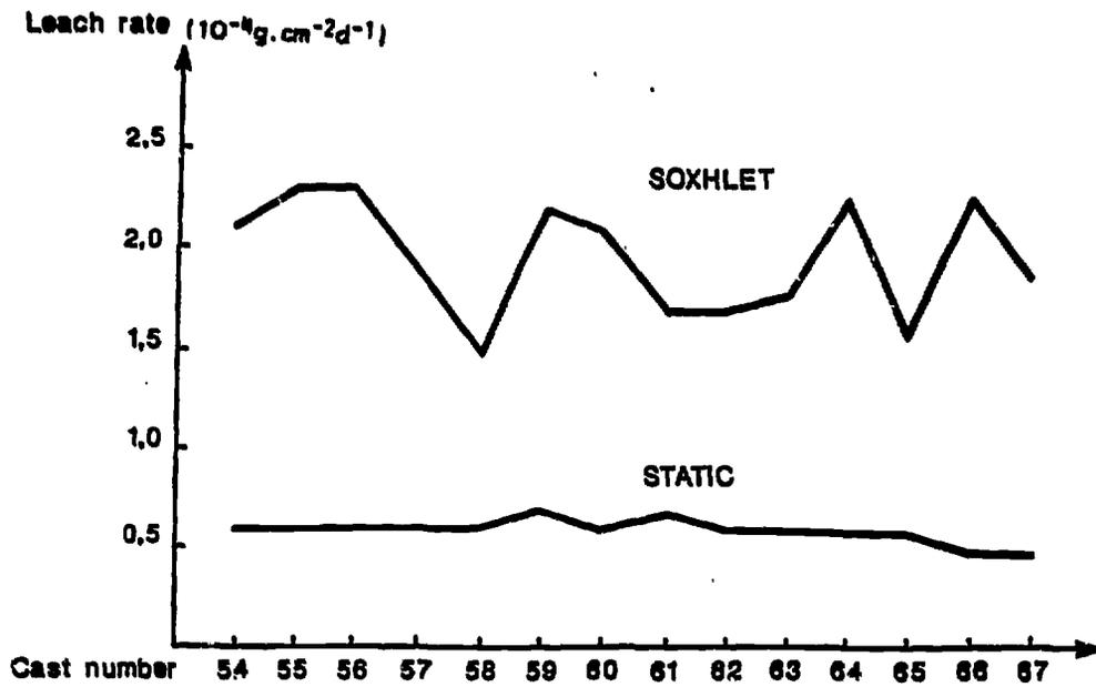
Fig. 6 : Modification of the leach rate versus time (14 consecutive casting operations) of a non radioactive full scale glass
