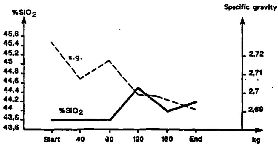
Fig. 3 : Modification of the specific gravity and of the SiO<sub>2</sub> content of a non radioactive full scale glass during the pouring
