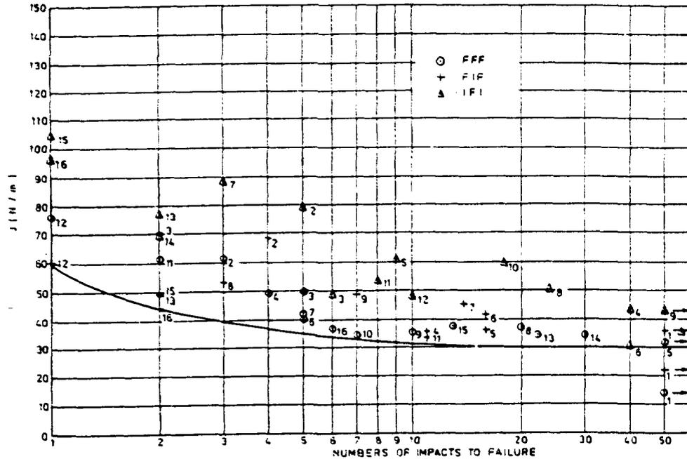
FIG. 13. Impact damage endurance curve.
