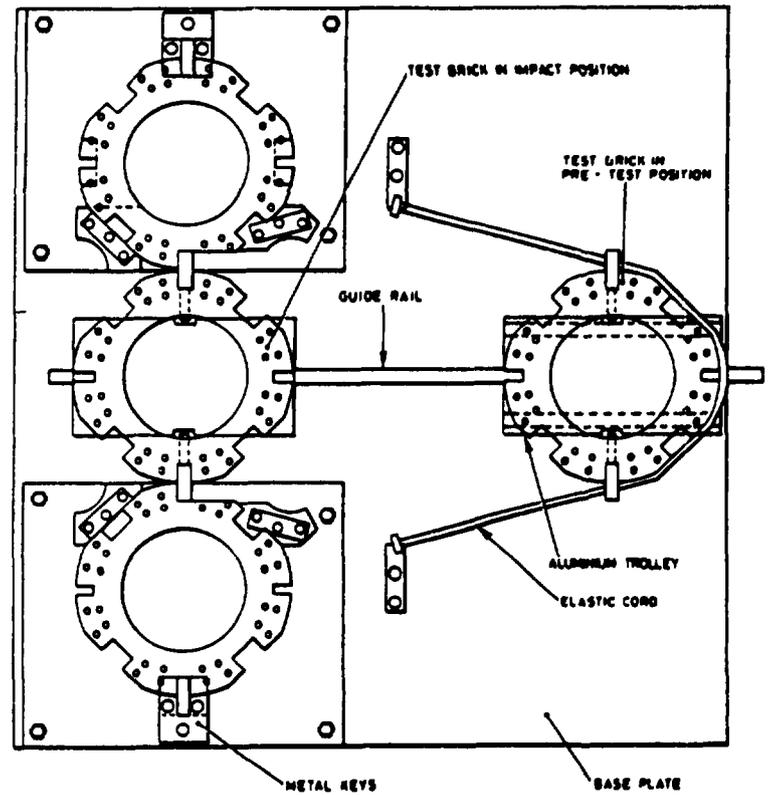
FIG. 12. Impact damage test rig.
