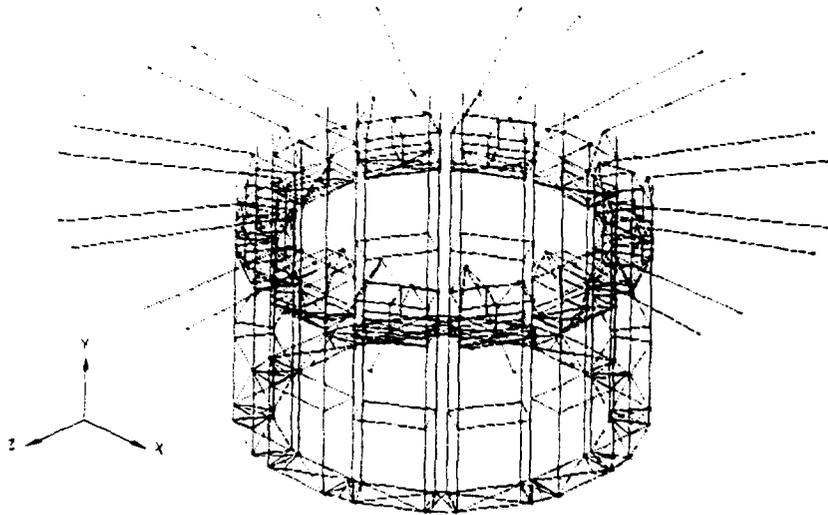
FIG. 4. FE model of boiler ring.
