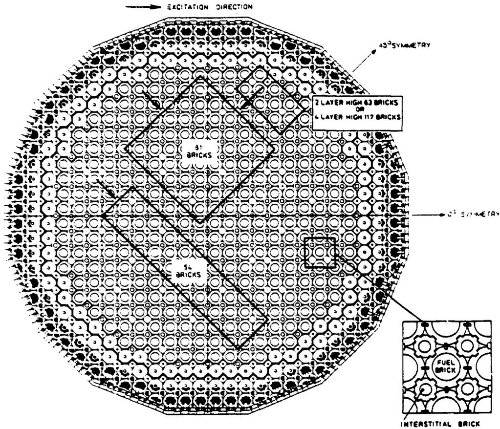
FIG. 7. Comparison between the brick test arrays and a core brick layer.
