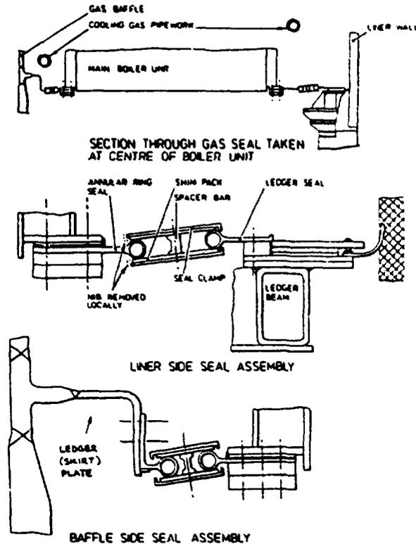
FIG. 3. Arrangement of main boiler gas seal.
