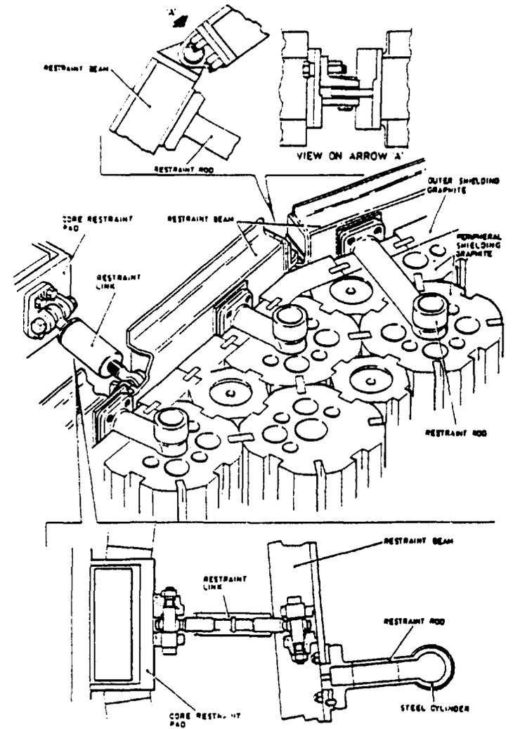
FIG. 8. Arrangement of restraint system.
