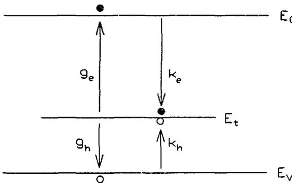
Fig. 5. Schematic of electron and hole capture and emission processes between the level  $E_t$  and the conduction and valence bands.
