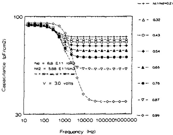
Fig. 8. Calculated C-f plots as a function of  $N_{t1}/N_{t-d}^{-d}$ .
