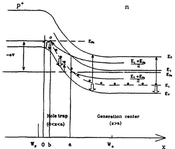
Fig. 6. Illustration of the charge states of a deep acceptor-like center in the band gap. The center is occupied in the majority portion of the junction and acts as a compensation center.
