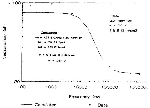
Fig. 10. Comparison between calculated and measured C-f data.
