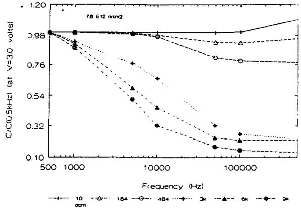
Fig. 3. Data of detector capacitance (at 3.0 V) vs frequency as a function of Si resistivity.
