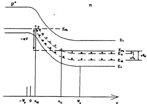
Fig. 4. Energy band diagram for the proposed two-level model describing the observed frequency-dependent C-V effects.
