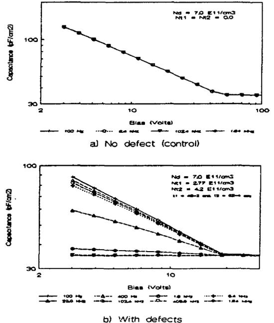
Fig. 7. Calculated frequency-dependent C-V characteristics with a) No defects (control); and b) two defect levels.
