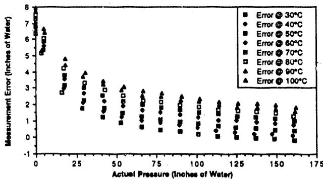
FIGURE 2. Sensor Pressure and Temperature Response
