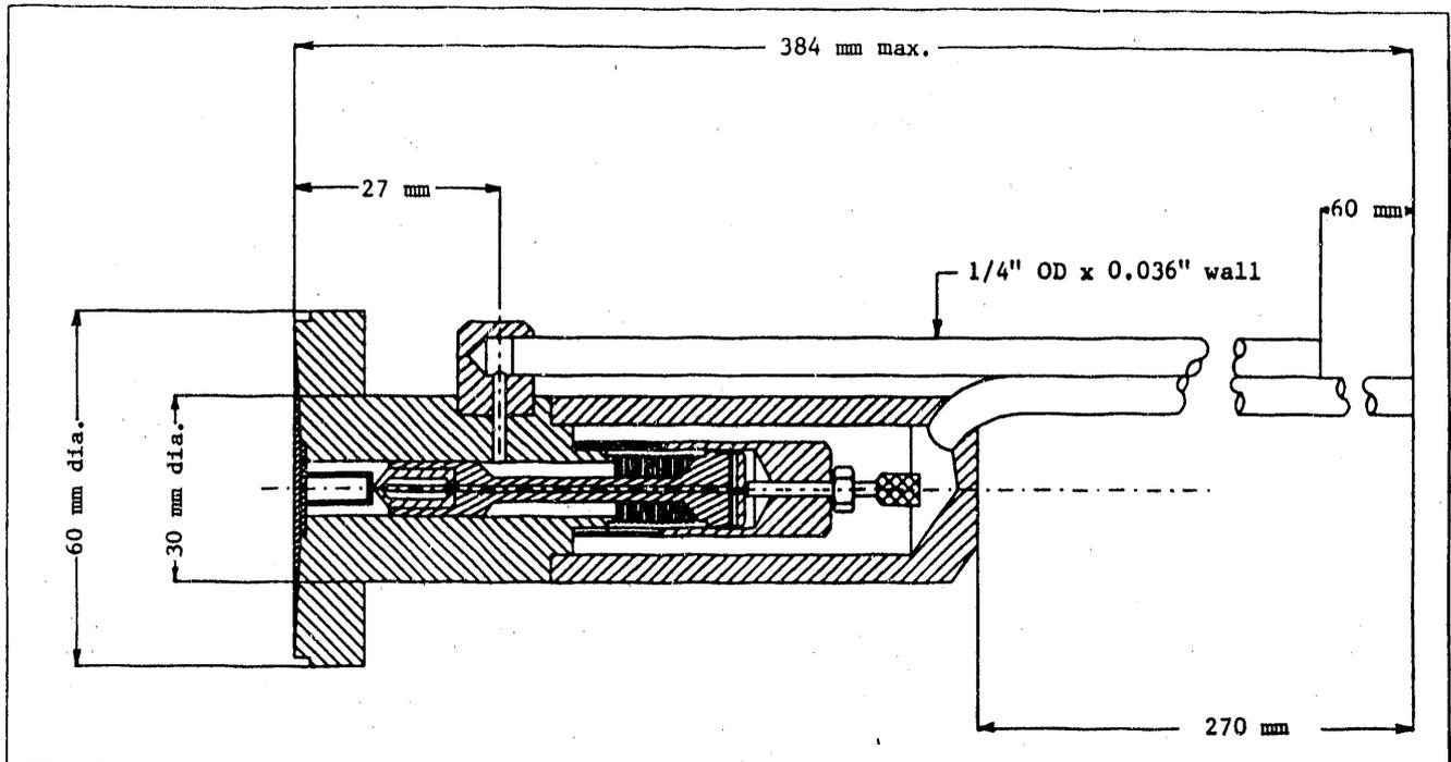
FIGURE 1. Sensor Detail
