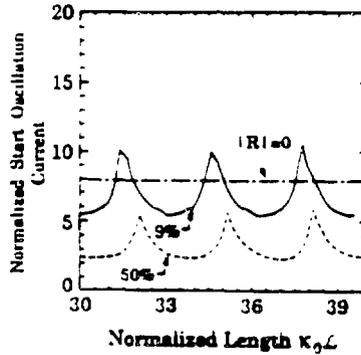
Figure 3: Normalized start oscillation current vs normalized length
