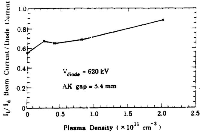
Figure 2: Beam current/diode current vs plasma density
