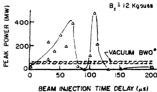
Figure 4: Peak microwave output power vs beam injection time delay
