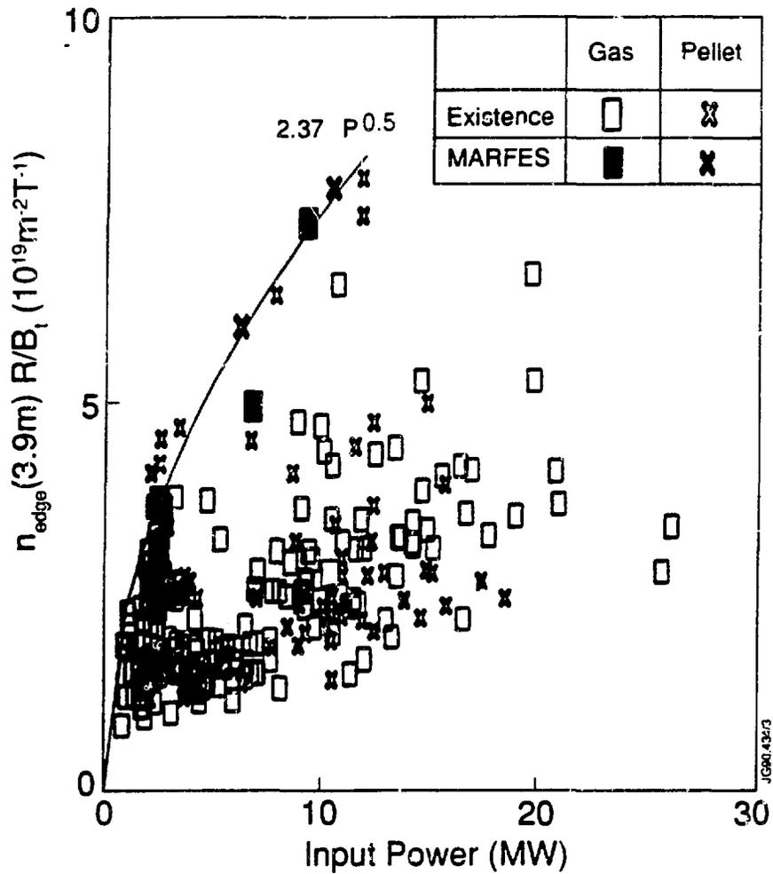
Fig.2. The normalised edge density versus input power showing that the MARFE density limit occurs at the boundary of the existence region close to the curve  $n_{edge} R/B_1 = 2.37 P^{1/2}$  [ $10^{19} m^{-3}$ , m, T, MW].  $B_1$  varies in the range 1.4 to 2.6 T.
