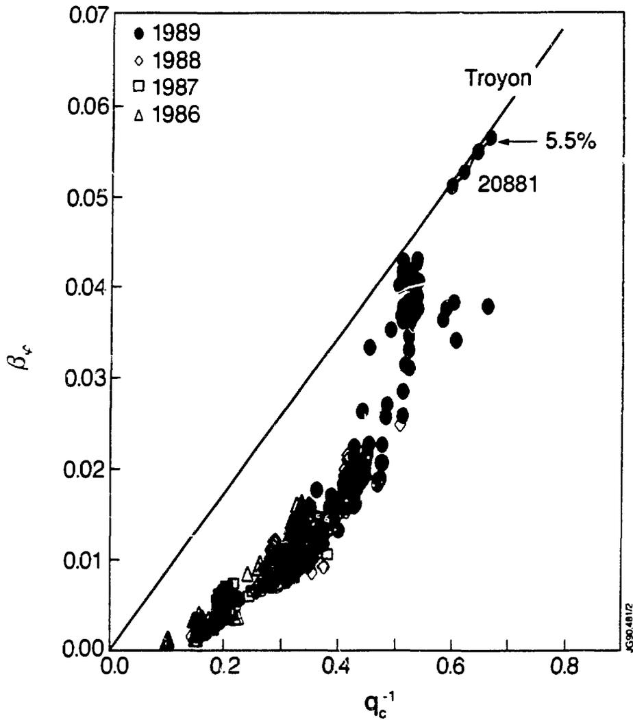
Fig.3. The maximum toroidal beta ( $\beta_c = 2\mu_0 \langle p \rangle / B_p^2$ ) as a function of  $q_c^{-1}$  (proportional to normalised current  $I_p / B_p a$  [MA, T, m]), for all JET discharges with the poloidal beta  $\beta_p > 0.4$ . The line is the Troyon limit  $\beta_{Troyon} = 0.028 I_p / B_p a$  [MA, T, m]. The highest  $\beta$  is 5.5%.
