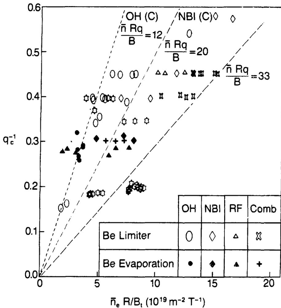
Fig.1 The operating density range for JET shown as normalised current  $q_c^{-1} = \pi R I_p / 5 A B_0$  [m, MA, m<sup>2</sup>, T] versus normalised density  $n_e R/B_t$  [ $10^{19}$  m<sup>-3</sup>, m, T]. Comparison is made between carbon disruptions (two broken lines at left) and MARFES with Be evaporation (solid symbols) and Be limiter (open symbols)
