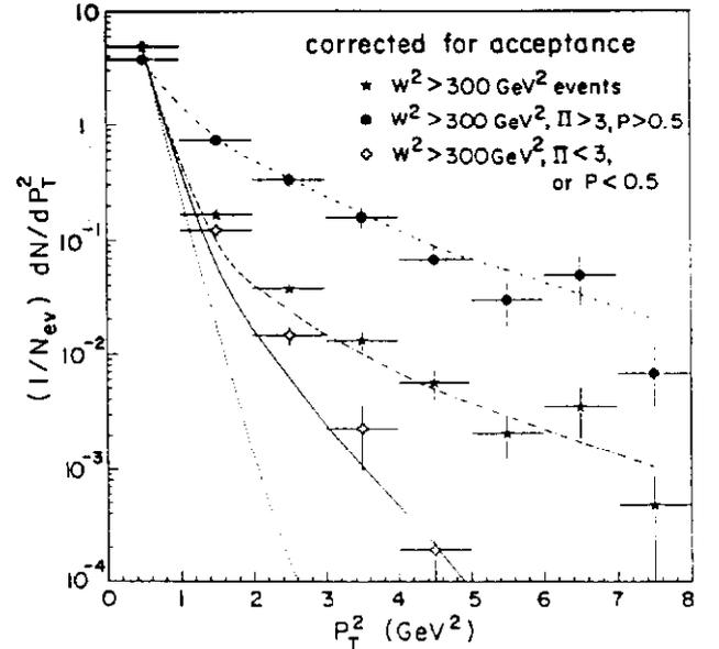
Figure 5: The average charged particle multiplicity per unit  $P_T^2$  for  $n_{ch} \geq 4$ .
