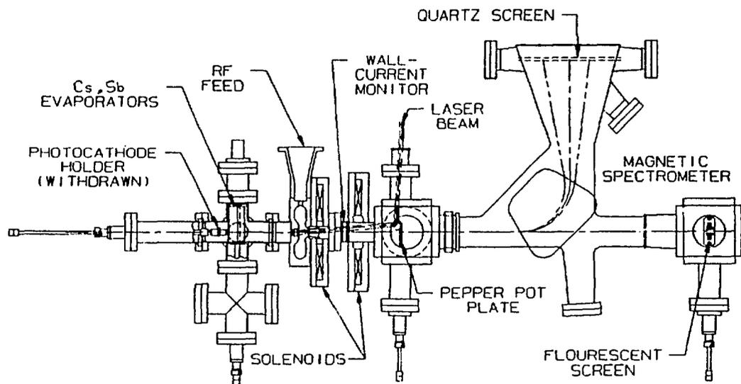
Fig. 10: LANL photo-injector set-up (from reference 55)
