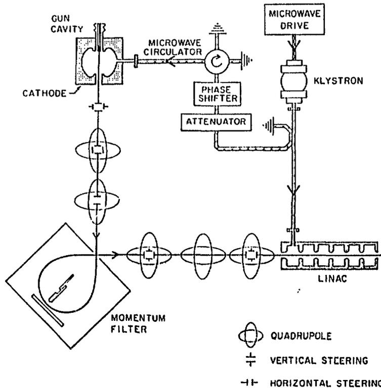
Fig. 8: Thermionic RF gun lay-out (from reference 41)
