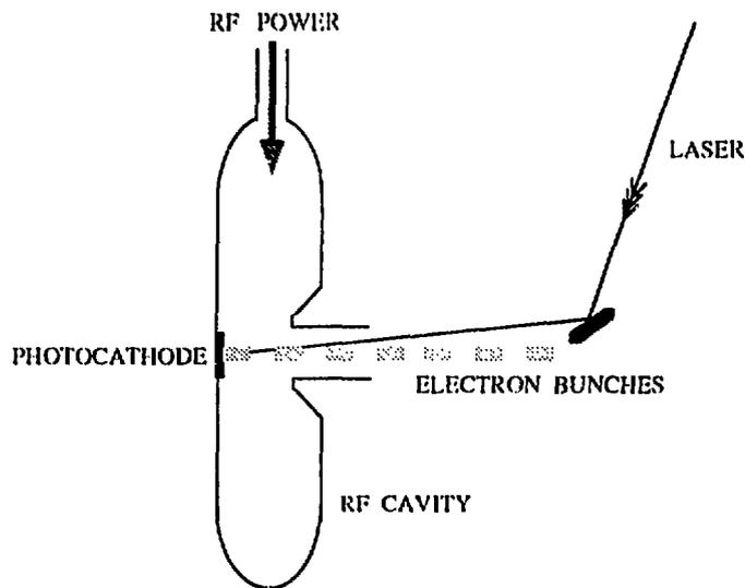
Fig. 9: Laser-driven RF gun
