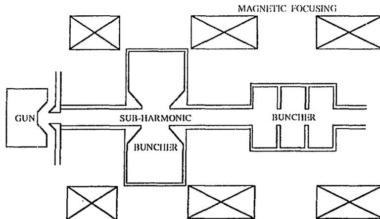
Fig. 3: Conventional injector
