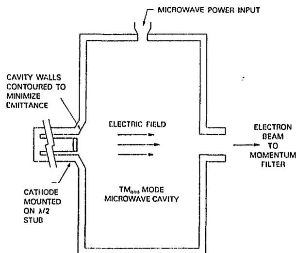
Fig. 7: Thermionic RF gun (from reference 36)
