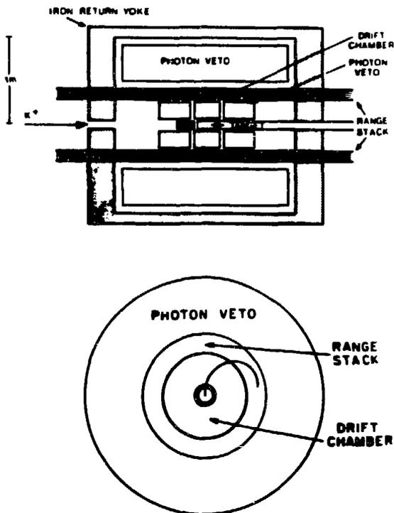
Fig. 4. Conceptual design of a kaon factory experiment to measure  $K^+ \rightarrow \pi^+ \nu \bar{\nu}$ .
