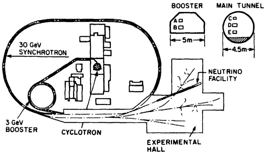
Fig. 2. Possible site layout together with cross sections through the tunnels
