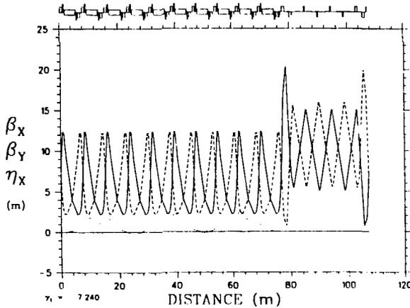
Fig. 2. Lattice functions of the racetrack Booster.
