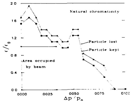
Fig. 4. Dynamic aperture in the Driver.
