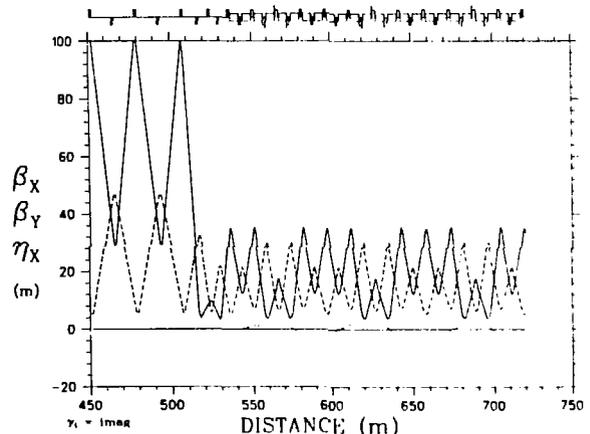
Fig. 1. Lattice functions of a racetrack Driver quadrant.
