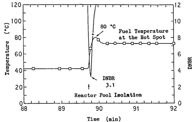
Fig. 10 DNBR and Fuel Temperature at the Hot Spot at the Flow Reversal (Primary Coolant Pipeline Break)
