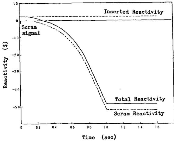
Fig.5 Inserted, Total and Scram Reactivity (Reactivity Insertion by Removal of In-core Irradiation Samples)
