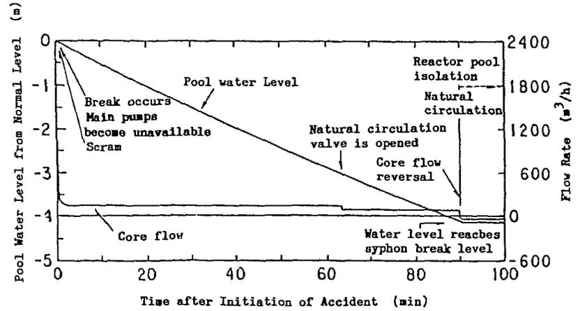
Fig.6 Transient of the Pool Water Level and the Core Flow (Primary Coolant Pipeline Break)
