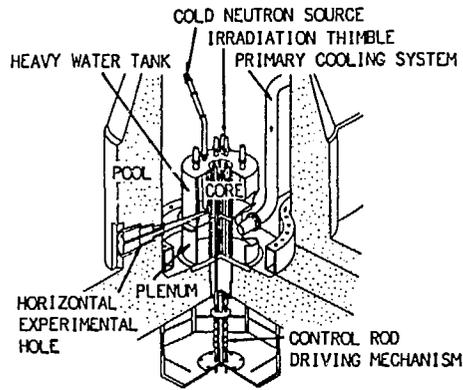
Fig. 1 Core components
