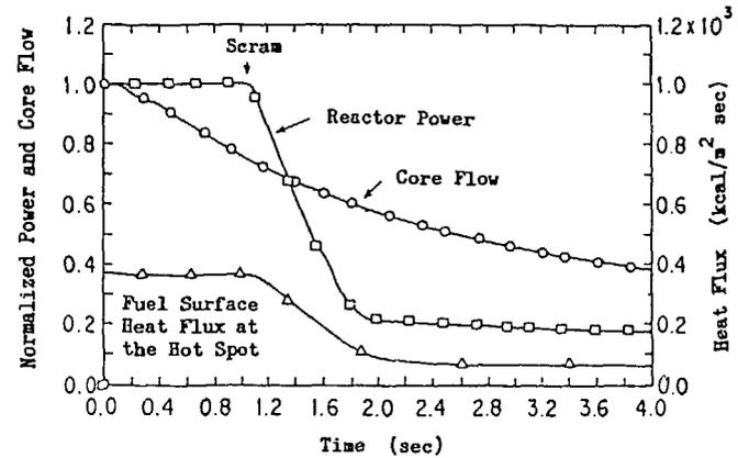
Fig.7 Normalized Power and Core Flow, and Fuel Surface Heat Flux at the Hot Spot (Primary Coolant Pipeline Break)
