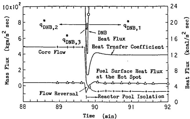
Fig. 9 Core Flow, Fuel Surface Heat Flux at the Hot Spot, Heat Transfer Coefficient and DNB Heat Flux at the Flow Reversal (Primary Coolant Pipeline Break)
