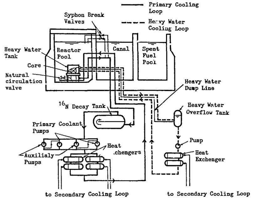
Fig.3 Schematic Diagram of Primary Cooling Loop and Heavy Water Cooling Loop
