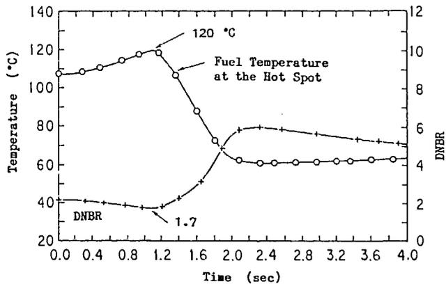
Fig. 8 Fuel Temperature at the Hot Spot and DNBR (Primary Coolant Pipeline Break)
