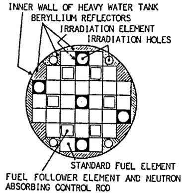
Fig. 2 Configuration of the core
