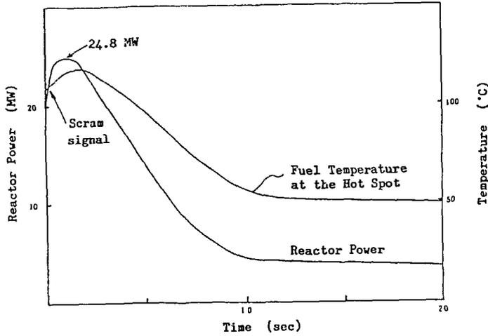
Fig.4 Reactor Power and Fuel temperature at the Hot Spot (Reactivity Insertion by Removal of In-core Irradiation Samples)
