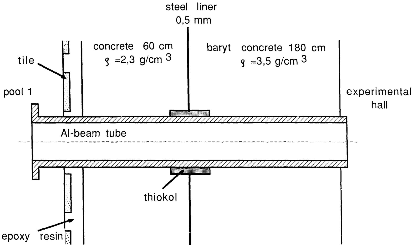
Fig. 3: Cross section of the biological shield
