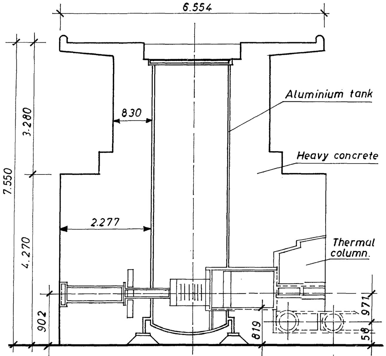
Fig.1 Vertical cross section of the C. R. E. N. - K. Reactor.
