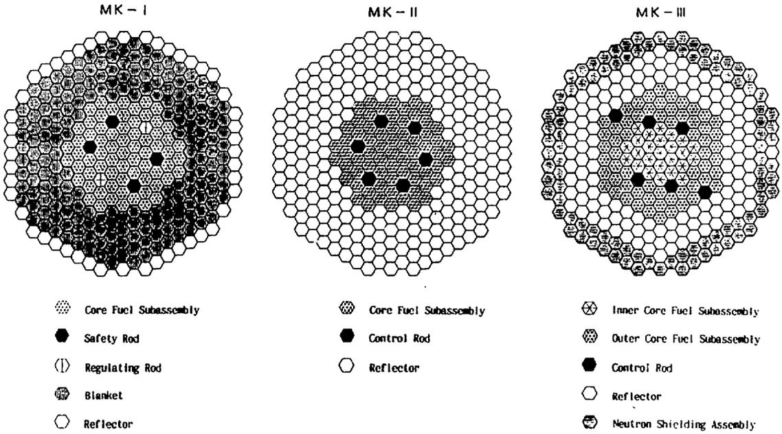
Fig. 3 Core Configuration
