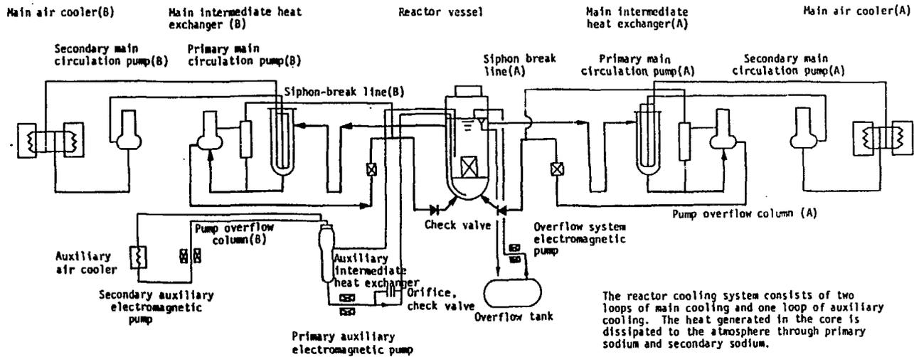
Fig. 2 Reactor Cooling System
