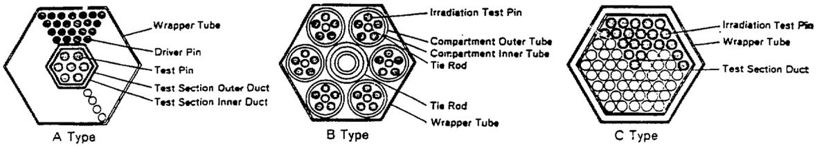
Fig. 4 Uninstrumented Irradiation Subassemblies
